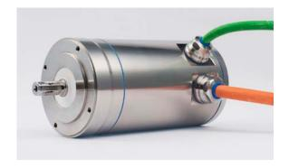
**Figure 6:** Motor H does not have any metal to metal joints. Instead, all joints are mated with gaskets. The gaskets are bright blue in color to contrast against food products.
