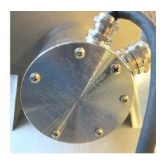
**Figure 2:** Motor C has a high-risk texture surface for product trapping and bacteria harboring. The uneven surface finish creates niches where microorganisms can hide.
