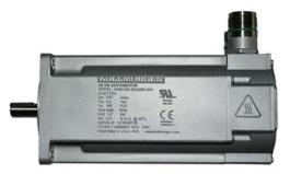
**Figure 1:** Motor *W* has an etched label covered with paint. The etching process creates a rough uneven surface that can create niches where bacteria and food product may be harbored.
