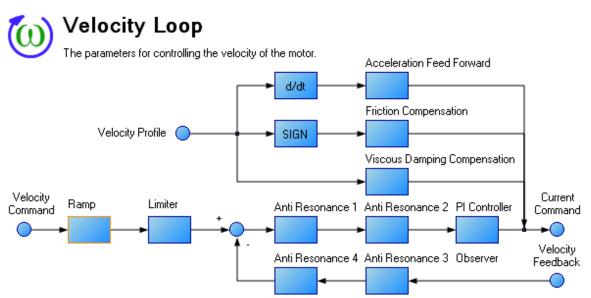
Figure 4 - Example of a highly-flexible servo loop from Kollmorgen's AKD servo drive family.
