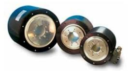
Figure 5 - Full frame DDR systems integrate all of the components of a complete motor, including the rotor, stator, bearings and feedback device, within a housing.
