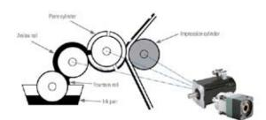
Figure 2 - In a "gearless" press configuration, each roller is driven independently by a motor/gearbox combination.
