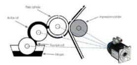
Figure 3 - In a direct drive press configuration, all rollers are driven independently by a direct drive rotary motor, without the need for gears or gearboxes.
