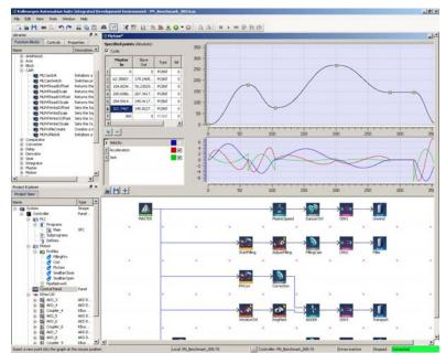
Integrated Development Environment showing Pipe Network<sup>TM</sup> and resident graphical CAM profile tool.
