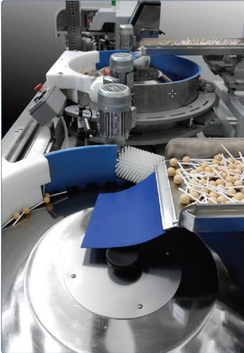
*About two dials, driven by KOLLMORGEN torque motors, the lollipops isolated and the packaging supplied.*
