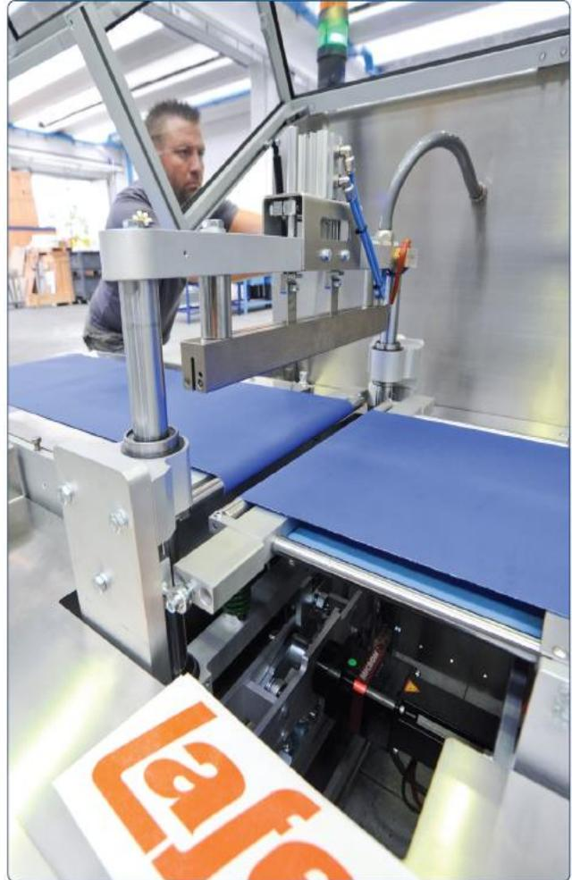
*KOLLMORGEN has supplied to the welding beam drive one recessed fully assembled motor-gear solution.*
