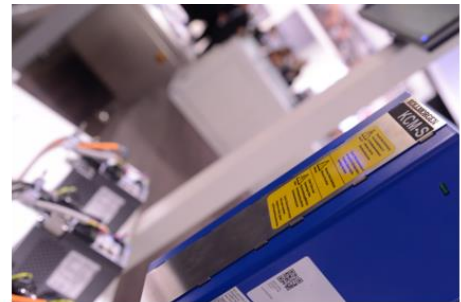
The KCM module increases energy efficiency with the flow of material as the braking energy can be used again for acceleration.
