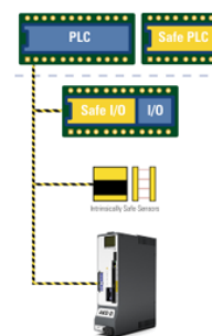
Safe FSOE communication for activating Safe Motion functions with the new AKD2G generation of servo drives saves considerable wiring effort. Availability also increases as some components and cables are known to improve overall system reliability..
