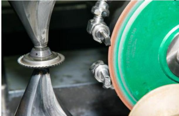
*The saw blades receive their last cut using a diamond wheel.*
