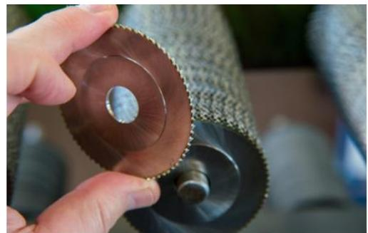
*Alesa has developed its own machine to grind the teeth on the circular saw blade.*
