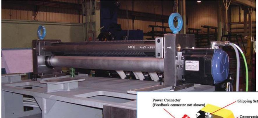
that support the roll also support the rotor. Feed accuracy is  $\pm 0.0005$ , an improvement over systems with mechanical transmission, with feed accuracy of 0.002.
