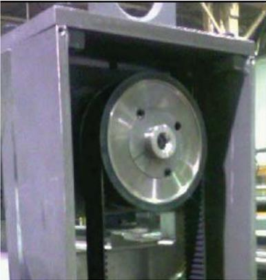
Above, a press machine uses a servomotor, gearbox, belt, and pulleys. The gear reducer decreases speed, increases torque, and also matches inertia between motor and load — a common approach. As the reflected inertia through a gearbox is reduced by the square of the gear ratio, a higher ratio reduces effective inertia seen by the motor.
