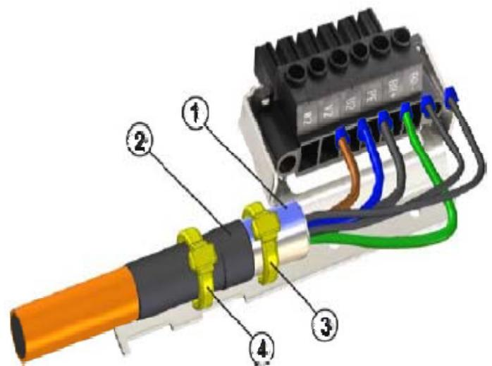
Wire the connector as show in the connection diagram and plug into the X2 socket on the front of the AKD. Screw the connector in place. This ensures that there is conductive contact over a large surface area between the braided shield and front panel.
