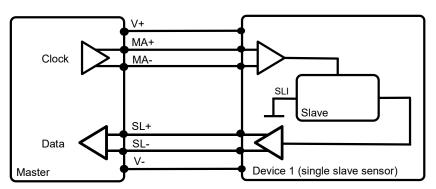
The Master transmits clock signals to the Slave via the MA line. The SL line carries the sensor data directly from the Slave back to the Master. The interface has only two unidirectional, differential lines (as the IncOder permanently connects the input SLI to '0'). Parameters for the individual data channels are specified below. These parameters can be pre-programmed in the controller and referenced via an ID or lookup table, or manually entered.
