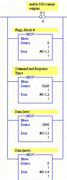
The command and data are now transmitted to the amplifier on each scan cycle, but the Data Handshaking protocol must be used to load the data. Wait for the command assembly to transmit, then set the Load Data bit high by writing 0x0001 to command word 0 (Output Word O:1.1). Now use the serial terminal to read the value of  $O_V - it$  should equal 1000.
