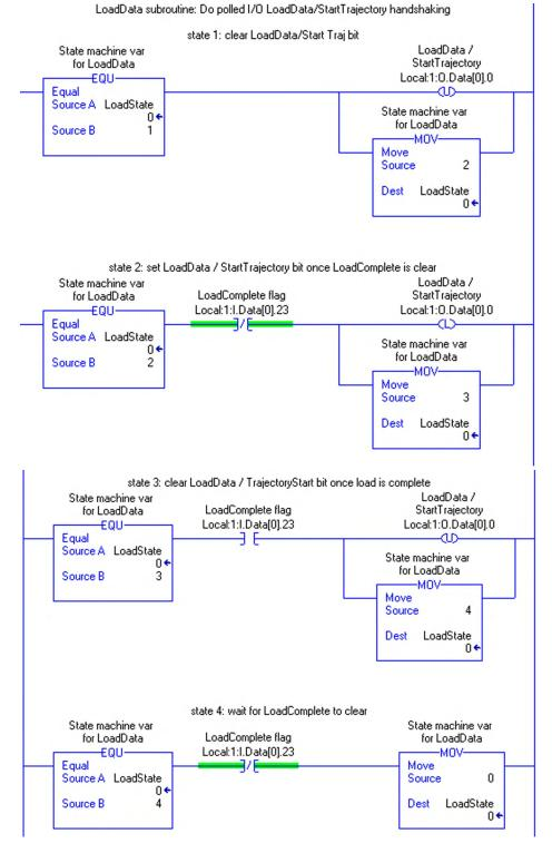
To use LoadData, first copy a proper command assembly into Local:1:O.Data[0-1]. Then set LoadState=1 and call the LoadData subroutine until LoadState has been reset to 0.
