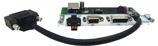
This chapter describes the Feedback extension card FB-2to1. The card enables simultaneous connection of a digital primary and of an analog secondary feedback to the connector X1. The supply of 24V DC auxiliary voltage to X33 is converted on the extension card into a precise 5V DC encoder supply for the secondary feedback.
