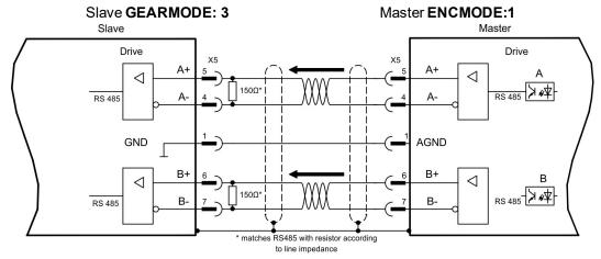
If SSI emulation is used, the master ENCMODE must be set to 2 and the slave GEARMODE to 5.
