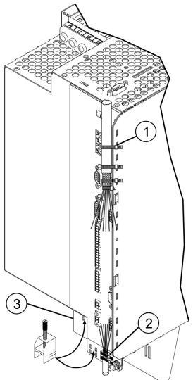
Remove the outside shroud of the cable and the shielding braid on the desired core length.
