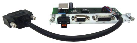
This chapter describes the Feedback extension card FB-2to1 for the S700. The card enables simultaneous connection of a digital primary and of an analog secondary feedback to the connector X1. The supply of 24V DC auxiliary voltage to X33 is converted on the extension card into a precise 5V DC encoder supply for the secondary feedback.
