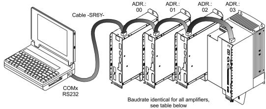
With the PC connected to only one amplifiers you can select every amplifier in the system via the set station address with the setup software.
