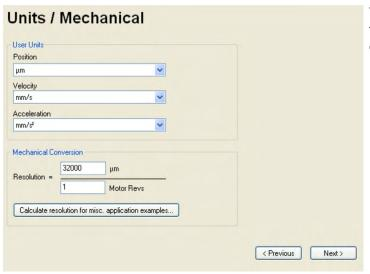
The user units for all input fields in the setup software can be preselected here.
