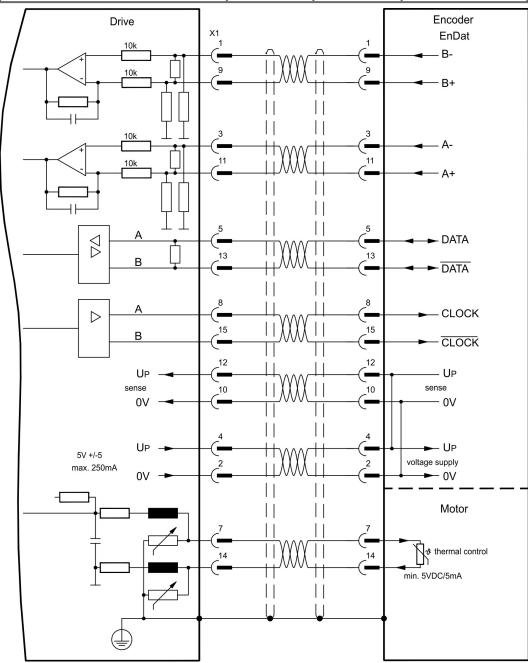
The pin assignment shown on the motor side relates to the AKM motors.  $\label{eq:control}$
