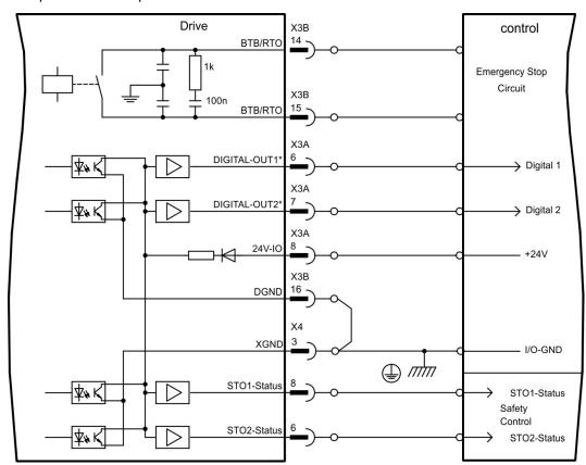
\* DIGITAL-OUT 1/2 must be defined as outputs using the setup software ("Digital I/O" screen page).
