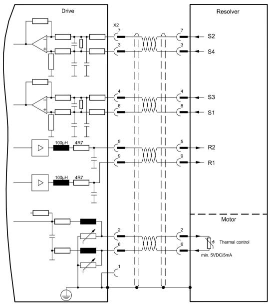
The pin assignment shown on the motor side relates to the AKM motors (connector code D).
