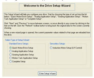
For a quick setup / drive test, select the setup type "Quick Motor/Drive Setup".
