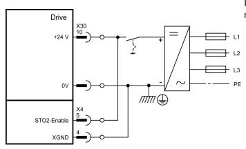
Input STO1-Enable [X4/7] must not be connected.
