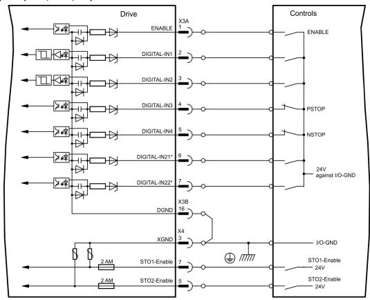
\* \* DIGITAL-IN 21 and 22 must be defined as inputs using the setup software ("Digital I/O" screen page).
