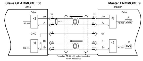
If using SSI emulation, then the master must be set to ENCMODE 10 and the slave to GEARMODE 25.
