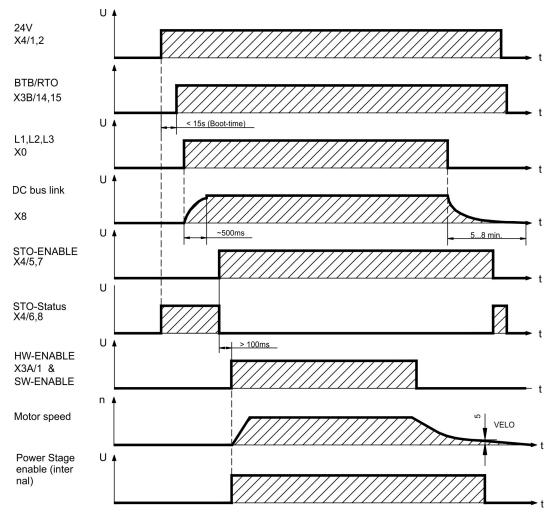
Devices which are equipped with a selected "Brake" function use a special sequence for switching off the output stage  $(\Rightarrow \# 33)$ .
