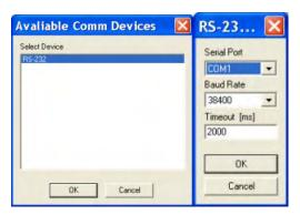
If the communication is started for the first time, you have to setup the communication parameters. Choose the communication system and the interface, where the servo amplifier is connected to. Click OK.
