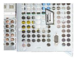
In the top of the servo amplifier there is a card reader for memory cards. The firmware and a full set of parameters (with control buttons and setup software) can be stored on the memory card and reloaded onto the servo amplifier.
