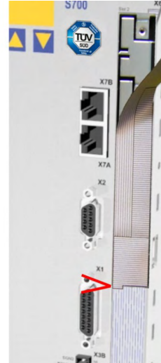
3 - Tear off the film (as far as the mark)
