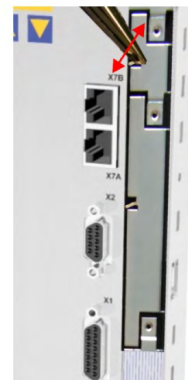
6 - Pull out the top plate
