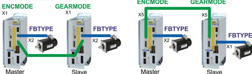
**Motor Feedback & Master Slave & External Position Feedback**
