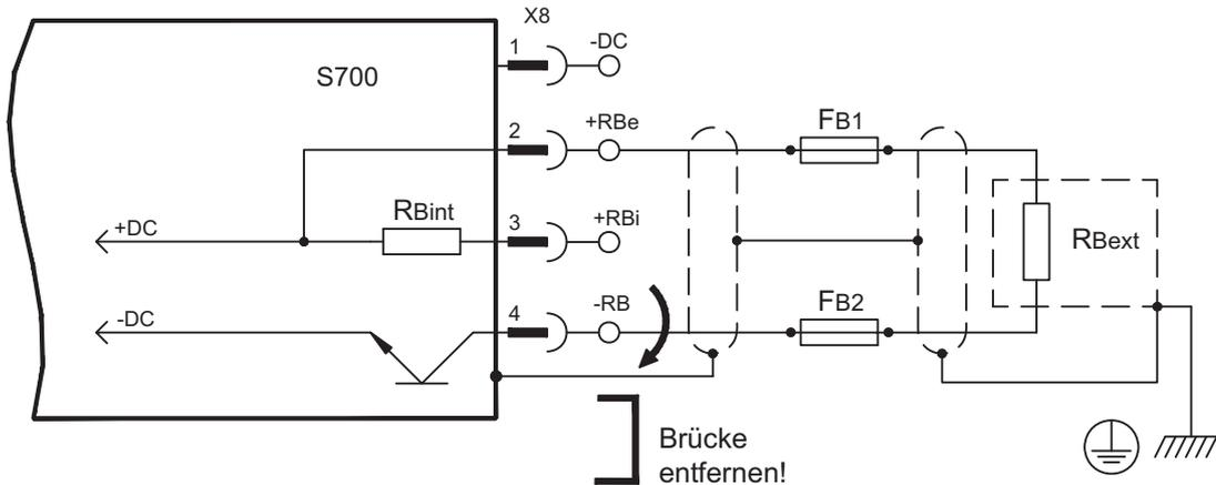
8.9.3 Kondensatormodule KCM (X8)
