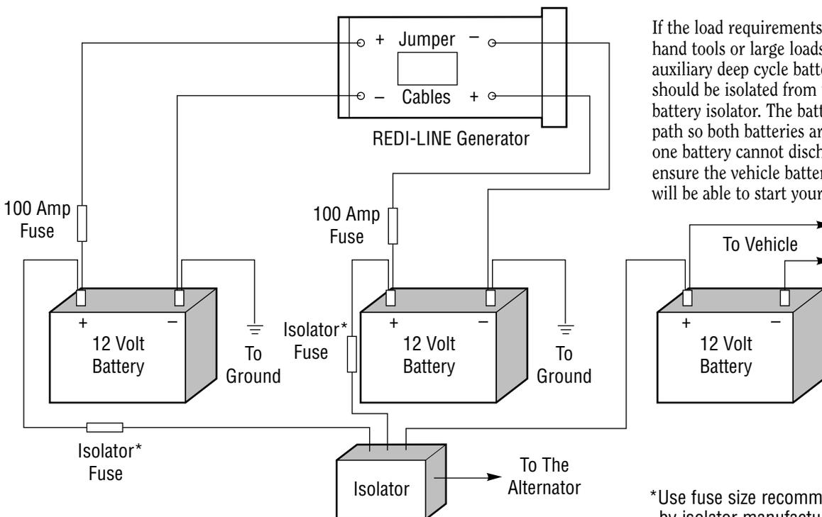
If the load requirements are heavy (constant use of hand tools or large loads) install two or more auxiliary deep cycle batteries. The auxiliary batteries should be isolated from the vehicle battery using a battery isolator. The battery isolator is a one way path so both batteries are charged by the vehicle but one battery cannot discharge the other. This will ensure the vehicle battery is always charged and you will be able to start your vehicle.
