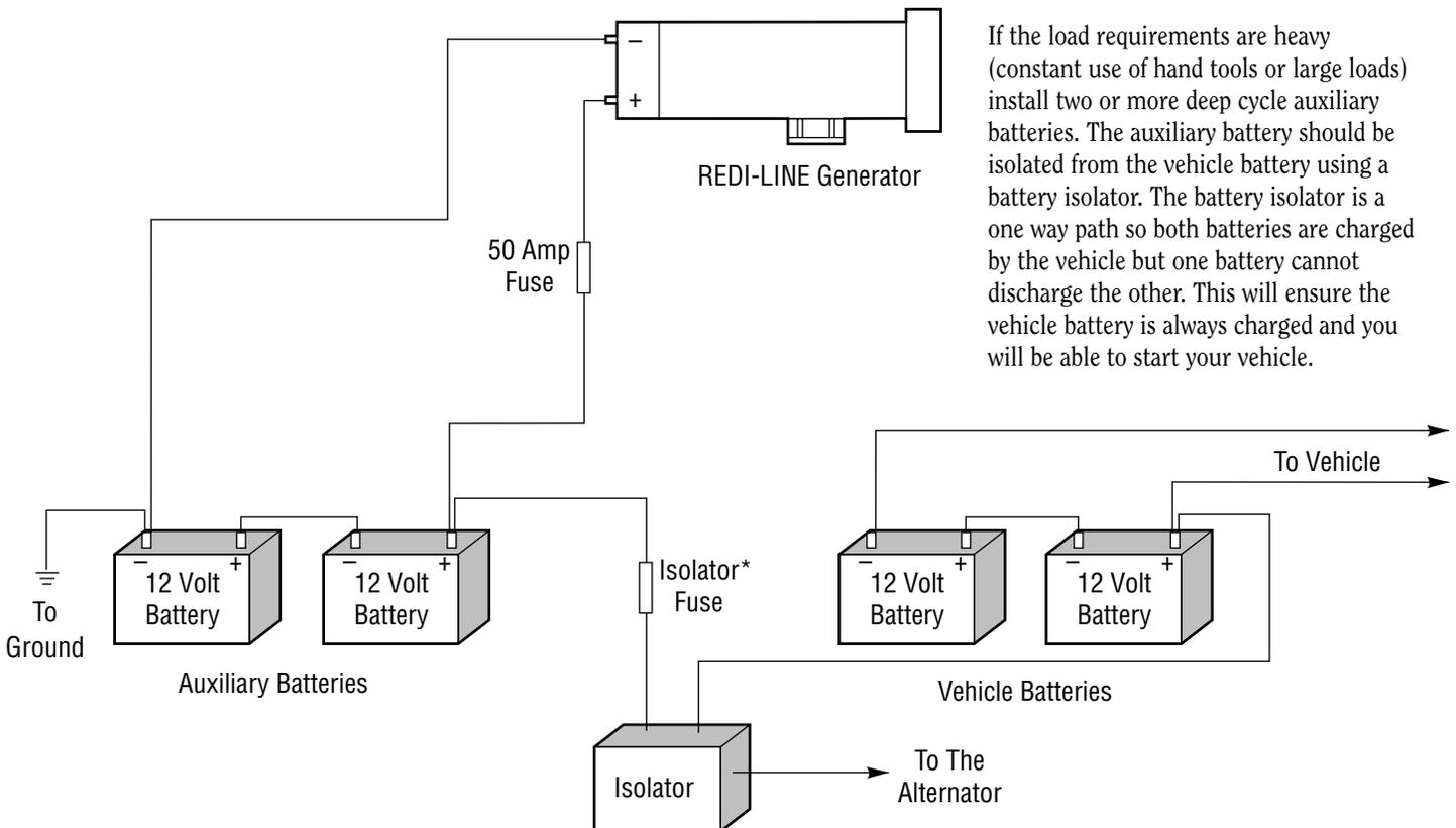
If the load requirements are heavy (constant use of hand tools or large loads) install two or more deep cycle auxiliary batteries. The auxiliary battery should be isolated from the vehicle battery using a battery isolator. The battery isolator is a one way path so both batteries are charged by the vehicle but one battery cannot discharge the other. This will ensure the vehicle battery is always charged and you will be able to start your vehicle.
