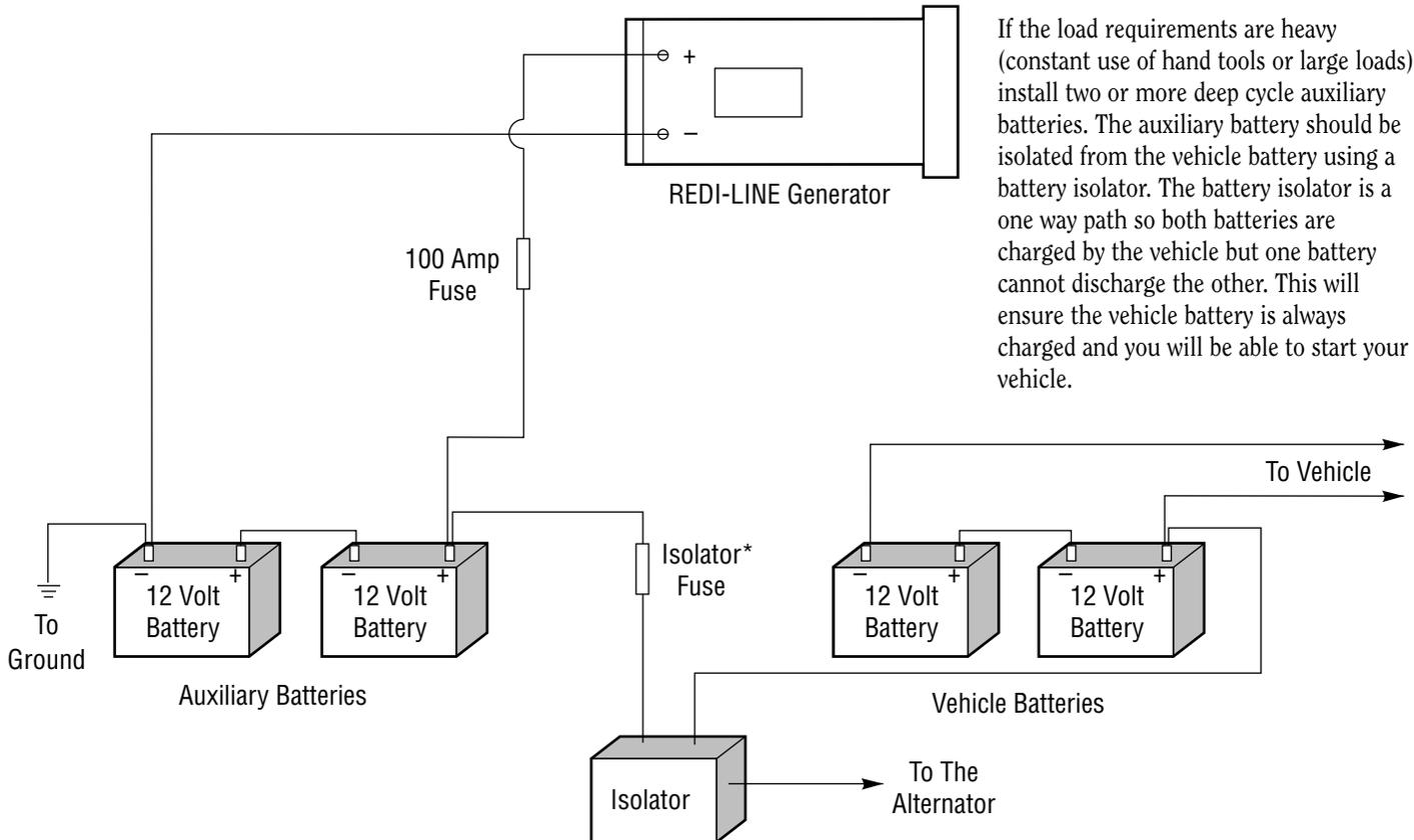
If the load requirements are heavy (constant use of hand tools or large loads) install two or more deep cycle auxiliary batteries. The auxiliary battery should be isolated from the vehicle battery using a battery isolator. The battery isolator is a one way path so both batteries are charged by the vehicle but one battery cannot discharge the other. This will ensure the vehicle battery is always charged and you will be able to start your vehicle.
