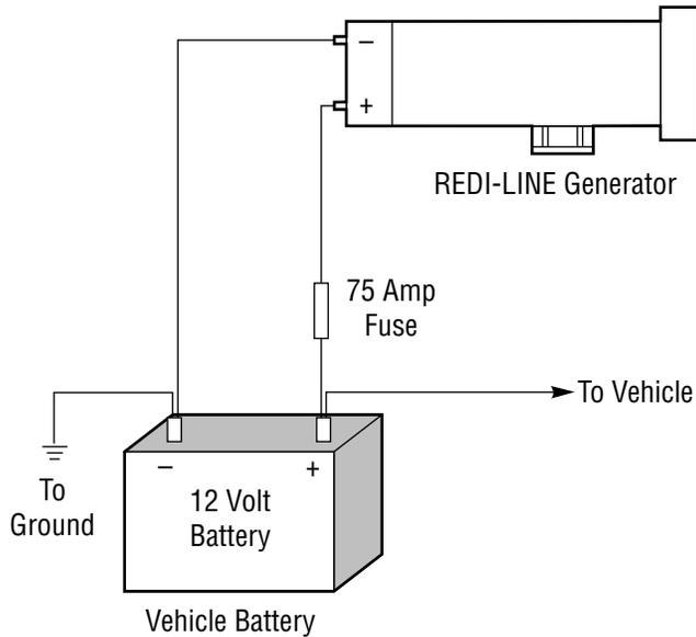
If the load requirement is not heavy (intermittent hand tool use or light loads for a long period of time) the vehicle battery and charging system should handle both vehicle and additional generator demand.
