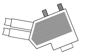
Use the strain relief to fix the cable to the bottom half of the housing. Do not overtighten the screws, or the cable will be crushed. Wire up the terminals according to the wiring diagram, and place the connector PCB with the terminals underneath in the lower half of the housing.
