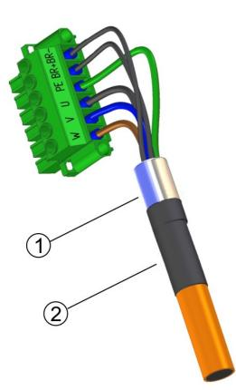
Strip the external cable sheath to a length of approximately 120 mm, taking care not to damage the braided shield. Push the braided shield (1) back over the cable and secure with a rubber sleeve (2) or shrink sleeve. Shorten all the wires apart from the protective earth (PE) wire (green/yellow) by about 20 mm so that the PE wire is now the longest wire. Strip all wires and fit wire end ferrules.
