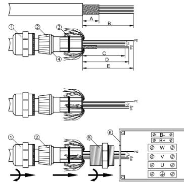
Preparing cables for terminal box, combined cables (AKM8, DBL7/8)
