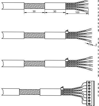
Remove the outer covering and the shielding braid over a length of about 100 mm. Remove another section of the outer covering, about 30 mm long, without damaging the shielding braid.
