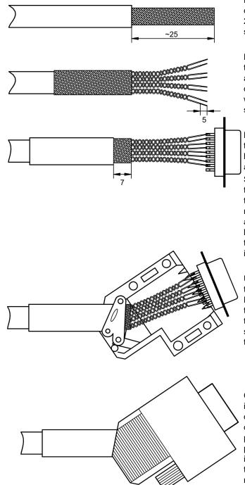
Remove the outer covering of the cable over a length of about 25 mm, without damaging the shielding braid.
