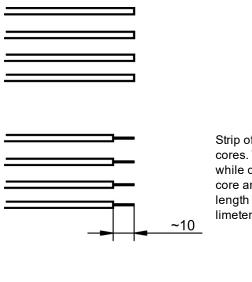
Strip off about 10 mm of the insulation at the ends of the cores. Take care to avoid damage to the copper strands while doing this. Depending on the cross-section of the core and the type of bootlace ferrule that is used, the length that has to be stripped may vary by several mil-limeters.
