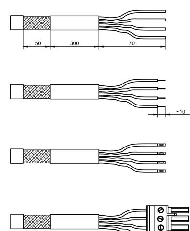
First, remove the outer covering of the cable and the shielding braid over a length of about 70 mm. Then remove just the outer covering for about another 50 mm, without damaging the shielding braid.
