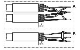
Remove the outer covering of the cable over a length of about 60 mm, without damaging the shielding braid.
