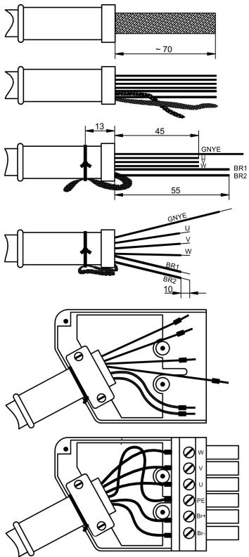
**First** push the rubber sleeve onto the cable, and **then** strip off about 70 mm of the outer covering, without damaging the shielding.
