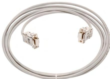
For the purpose of parameterisation and for firmware upgrades, the servo amplifiers can be connected to the serial RS232 interface on a PC. The connecting cable must be shielded. The braided shield on the RS232 connecting cable is conductively connected to the front panel of the servo amplifier via the connector housing on the Sub-D male connector.
