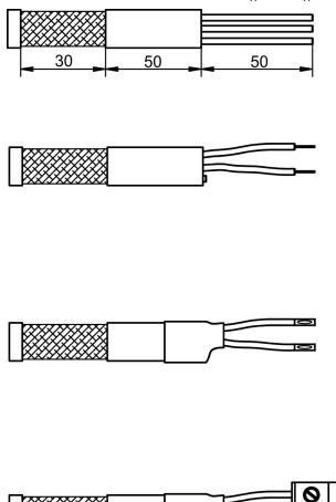
Remove the outer covering of the cable and the shielding braid over a length of about 50 mm. Then remove the outer covering without damaging the shielding braid.
