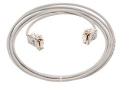
For the purpose of parameterisation and for firmware upgrades, the servo amplifiers can be connected to the serial RS232 interface on a PC. The connecting cable must be shielded. The braided shield on the RS232 connecting cable is conductively connected to the front panel of the servo amplifier via the connector housing on the Sub-D male connector.
