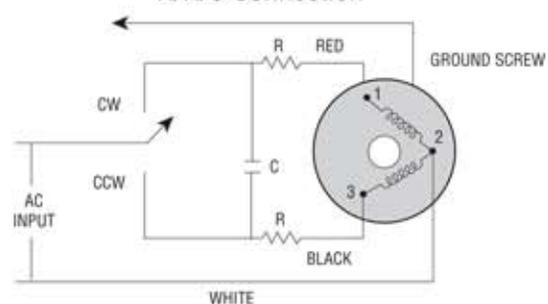
2 - Number in diagrams represent terminal connection when motors are supplied with terminal boards.
