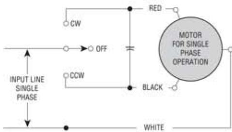
DIRECTION OF ROTATION DETERMINED WHEN VIEWED FROM NAMEPLATE END OF MOTOR.
