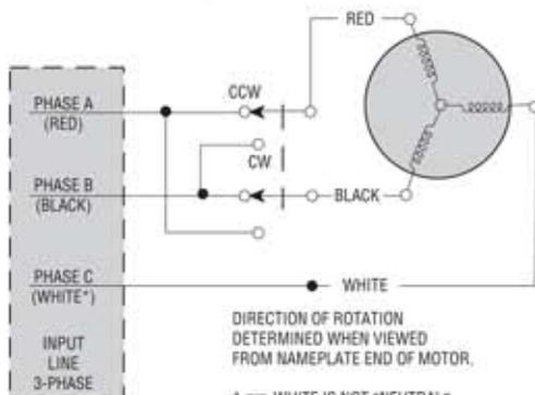
DIRECTION OF ROTATION DETERMINED WHEN VIEWED FROM NAMEPLATE END OF MOTOR.
