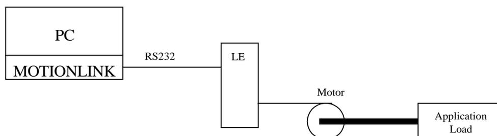
For system startup you need a PC with **MOTIONLINK** for windows, LE- CD-LITE drive brush less motor, and your application connected to the motor. With **MOTIONLINK**, you can initialize and configure you drive to your application. After that, you will connect the drive to your servo controller. You can communicate with the **SERVOSTAR** CD-Lite through the serial port.
