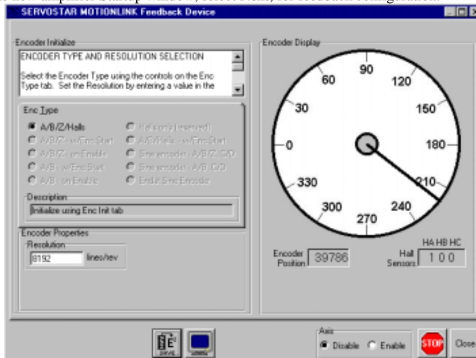
12. Select the encoder type and type the motor resolution in the resolution field (you can manually rotate the shaft for confirmation).
