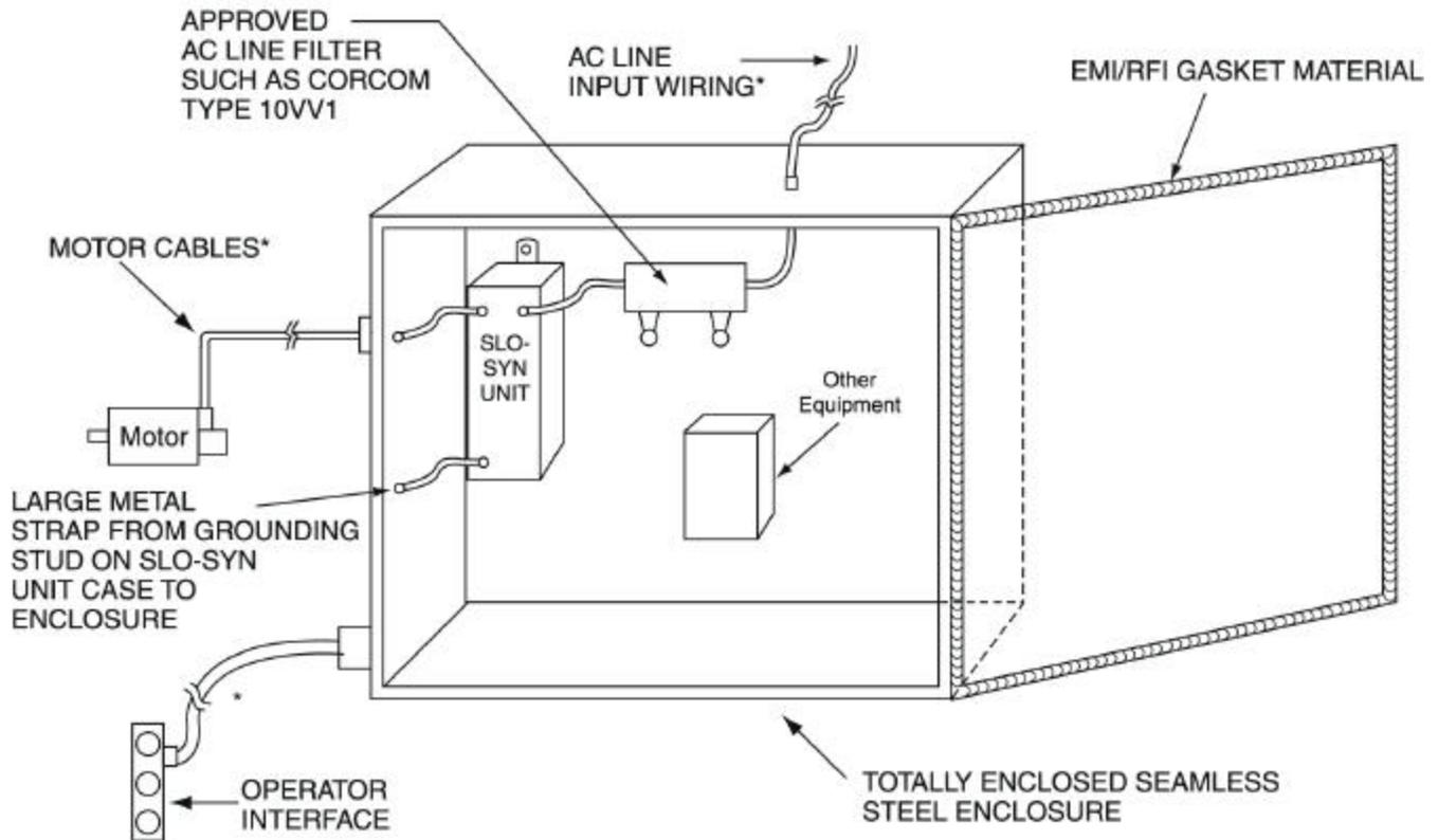
\* ALL WIRING RUNS THROUGH METAL JACKETED CONDUIT WHICH ARE ATTACHED TO ENCLOSURE WITH CLAMPS MAKING SOUND ELECTRICAL CONTACT.
