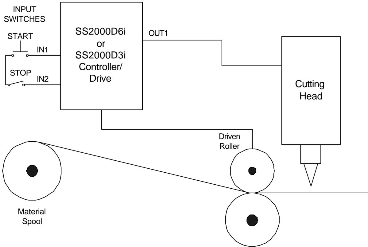
This application requires a stepper motor to run a pair of nip rollers that draw material from a spool. The material could be anything from paper to steel. The requirements for this application are:
