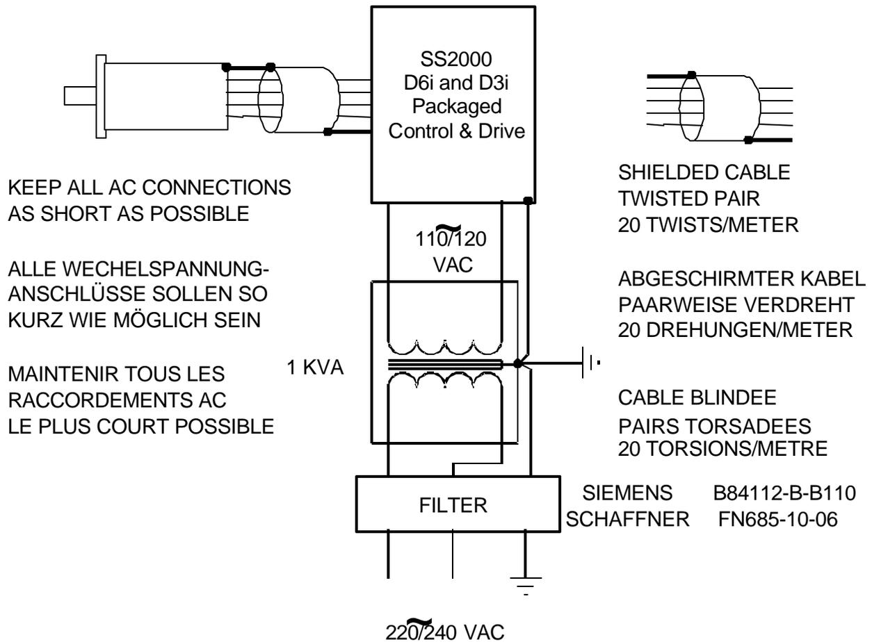
The following wiring practices should be used to reduce noise interference.
