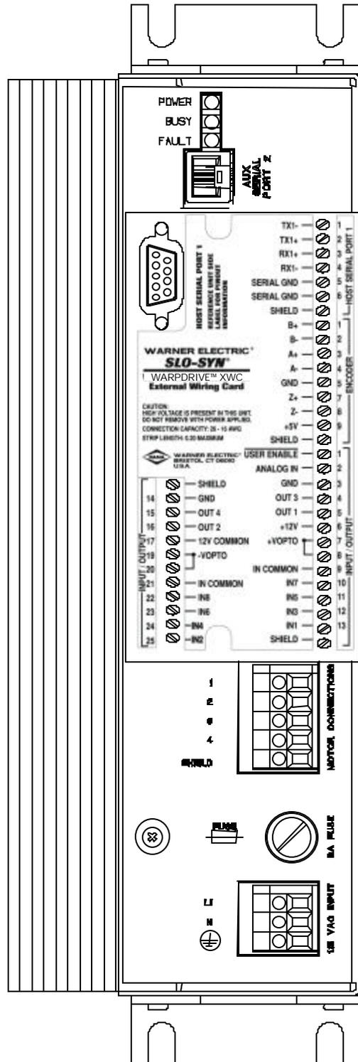
EXTERNAL WIRING CARD MOUNTED TO FRONT OF D6i or D3i UNIT
