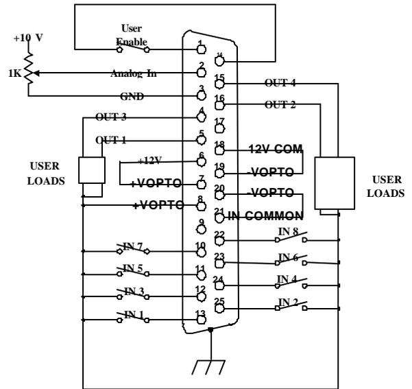
Depicted below are the I/O connections when using an External Power supply. Use these connections if you are not using the +12 Vdc internal power supply. The general purpose input connections are shown for both sinking and sourcing inputs.
