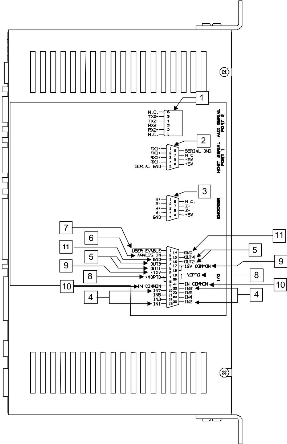
The following are brief descriptions of each connection to the D6i or D3i unit. More detailed wiring diagrams are provided in Section 3.5
