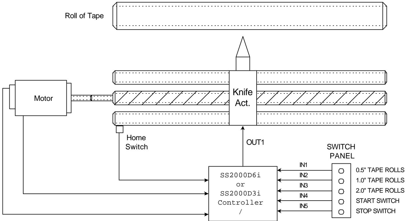
A manufacturer of adhesive tape uses a machine that takes a wide roll of tape and slits(cuts) it to the correct sizes. The program must be written to make tape widths of 2 inches, 1inch, and 0.5 inches from a 10 foot long roll. The size of the tape will be determined by the switch inputs from a switch selector panel. The machine will operate as follows:
