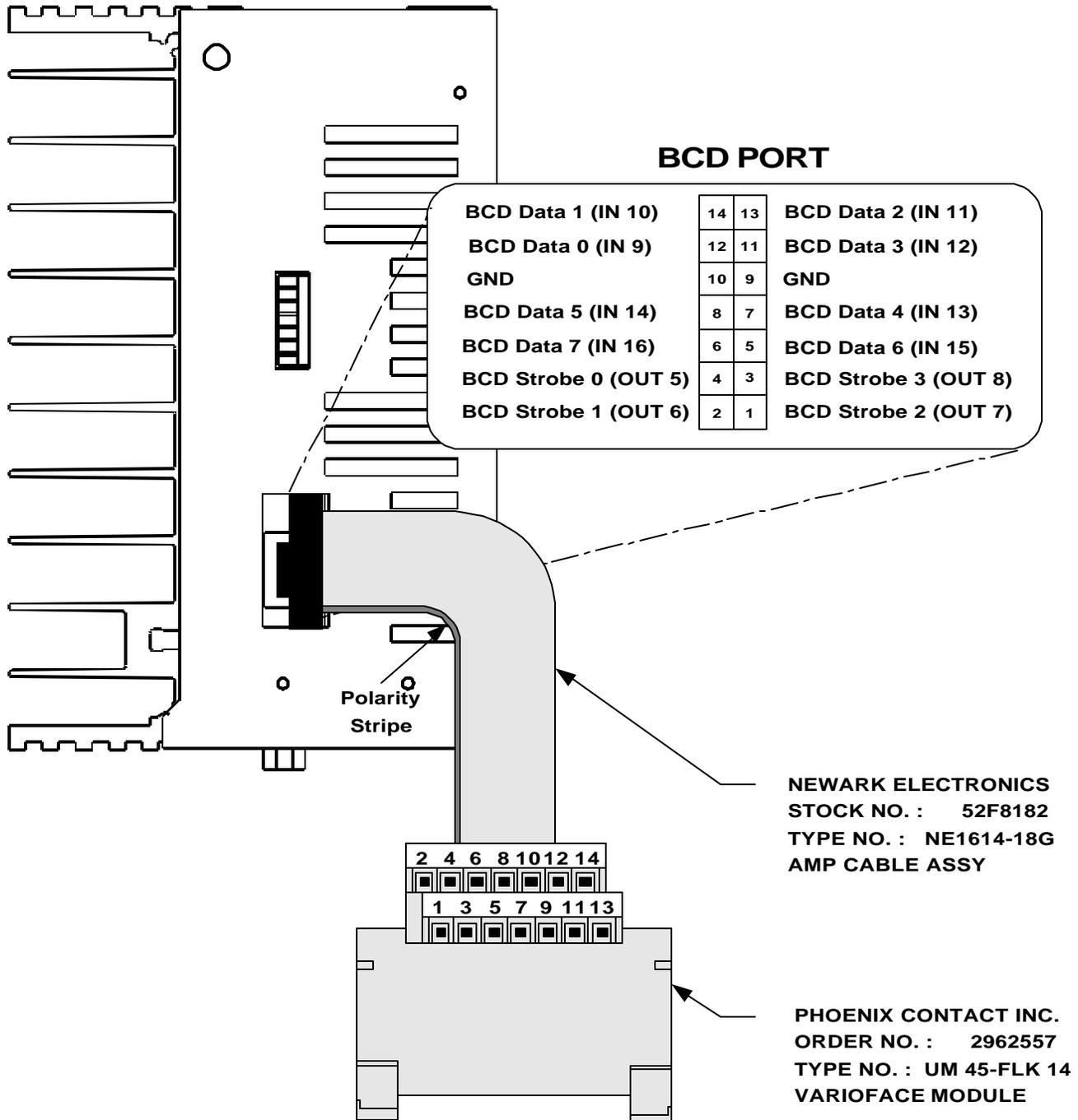
The connections for the BCD / TTL I/O connector when used as a BCD port are depicted below.
