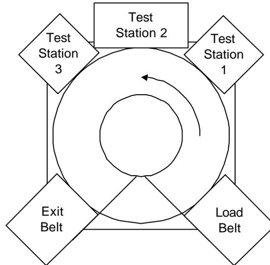
In this application, a part is loaded onto a rotary table via a load belt. Once the part is on the table, it must be tested at three test stations. The application requires:
