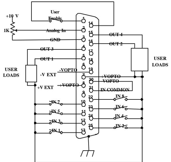
An optional external wiring card is available which provides individual terminals for each I/O point on the "D" style connectors utilized on the D6i or D3i unit. The External Wiring Card mounts over the D connectors on the face of the unit. All connections are brought out to individual clamp down type terminal connections. The
