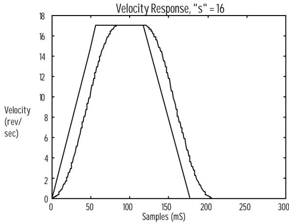
**Max. acceleration** sets the maximum allowed acceleration or deceleration rate in units/second<sup>2</sup>. This value is also used to decelerate motion to a stop when a fault such as a travel limit occurs.
