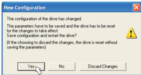
Parameters are uploaded to the amplifier's RAM now (takes some seconds). When this is done, you have to accept the changed configuration with "Yes" or to discard the changes in the appearing screen.
