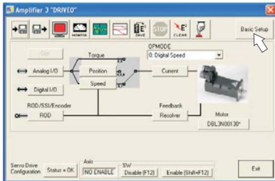
**Make sure, that the amplifier is disabled (Input HW-Enable connector X3 pin 15 must be 0 V or open)!**
