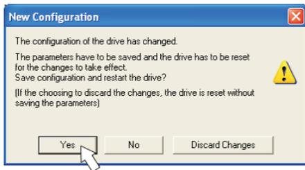
A warning appears, that you have to restart the amplifier. This is called "coldstart". Click "YES". The parameters are saved to the amplifier's EEPROM automatically and a reset command restarts the amplifier (takes a few seconds). For example, this happens after motor or feedback selection.
