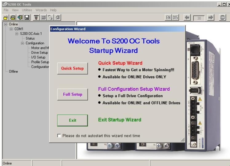
The first step is to confirm that the drive is configured for the motor being used. This information is automatically gathered from a system using an 'SFD-Equipped' AKM-Series motor.
