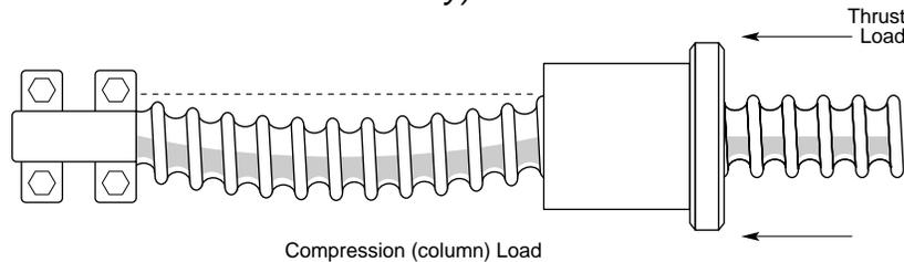
All leadscrews have a column loading limit which causes the screw to buckle or bend as thrust load increases. This limit is a function of unsupported leadscrew length. Exceeding this limit will cause the leadscrew to buckle and become permanently damaged.
