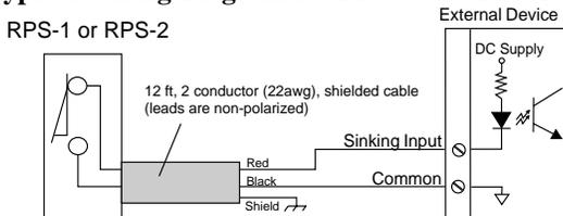
Typical Wiring Diagram for RP1 and RP2
