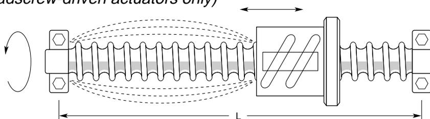
Leadscrew-driven actuators are speed-limited by the *critical speed* (also called the natural resonant speed) of the leadscrew. This speed is a function of actuator stroke length and leadscrew diameter. Operation at or above the critical speed limit can cause the leadscrew to bend permanently, resulting in low performance and noisy operation.
