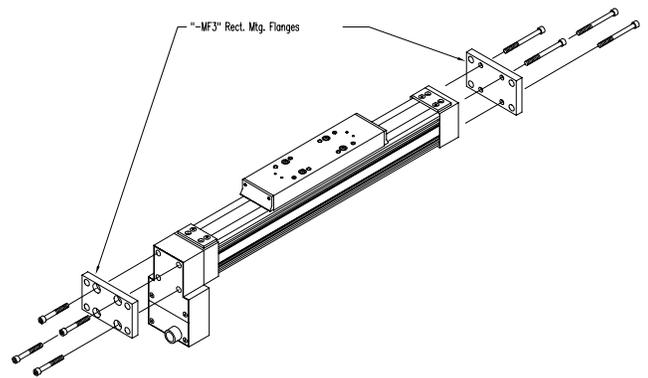
*Note:* Fasteners screw into blind hole. Do not use a fastener that protrudes more than 0.31 inches [7.8mm] into tapped hole.
