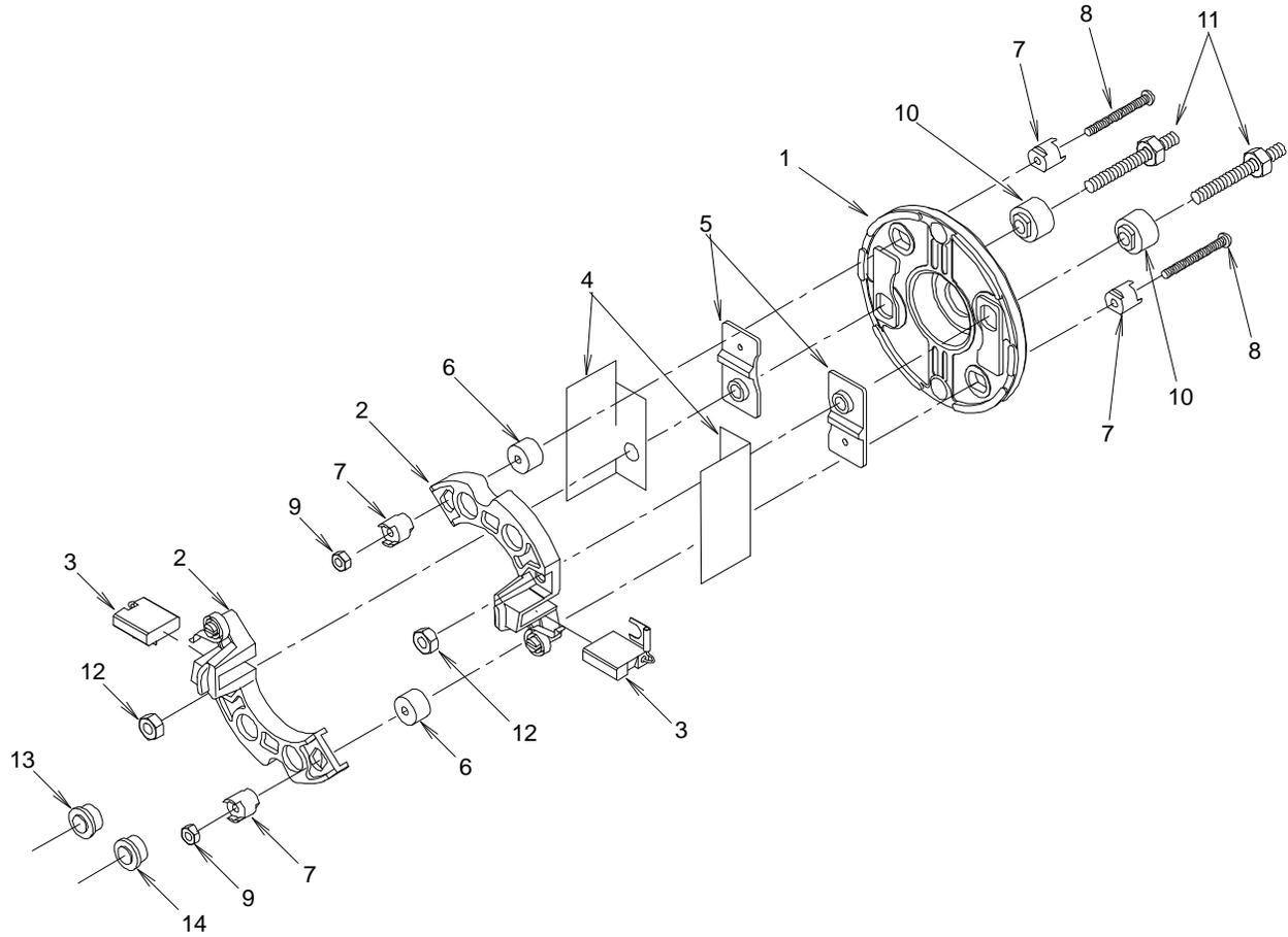
Figure 10-2. End Bell for Earlier Small Frame Generators
