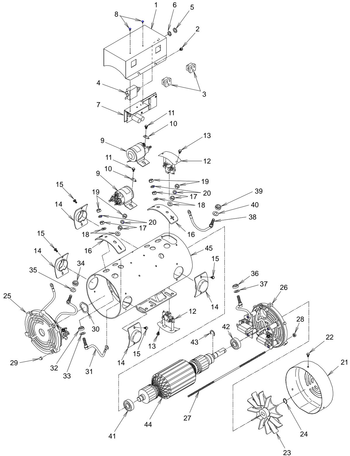
Figure 10-6: 12-Volt Large Frame Generator, Current Version, continued
