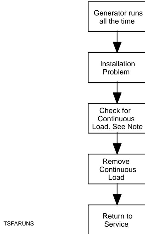
Note: Power strips with ON indicator lamps, equipment with POWER CONNECTED indicator lamps, or similar devices can place enough load on the generator to cause it to run, even though the intended load has been removed.
