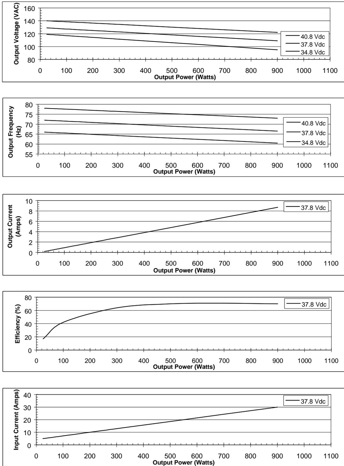
Figure 11-5: Performance Curves for DA36A-900A Redi-Line Generators
