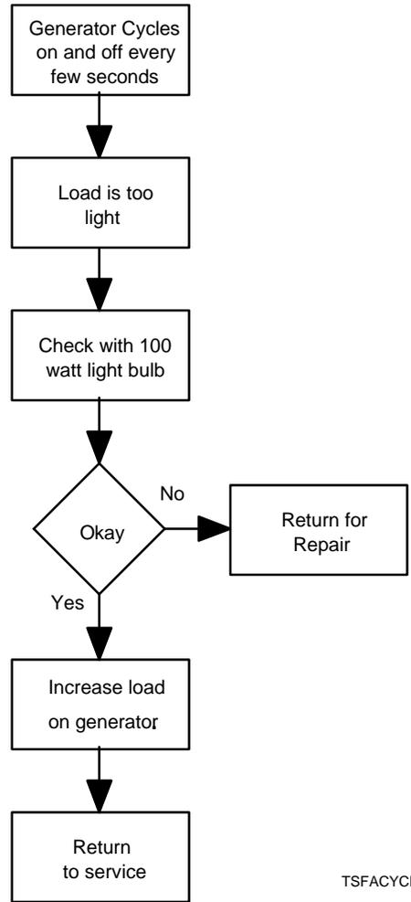
Figure 7-8. Generator Cycles On And Off Every Few Seconds
