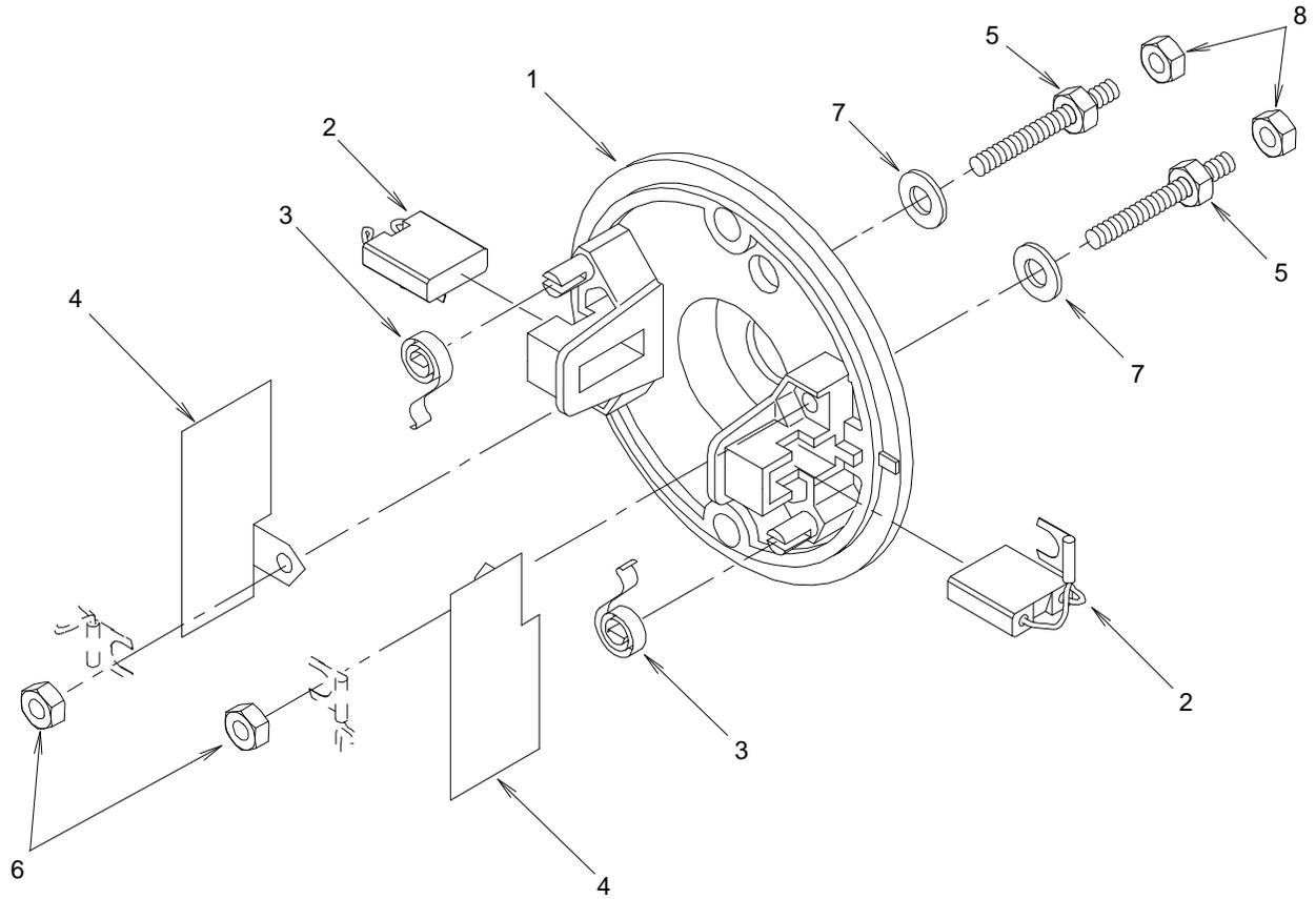
Figure 10-3. End Bell for Current Small Frame Generators
