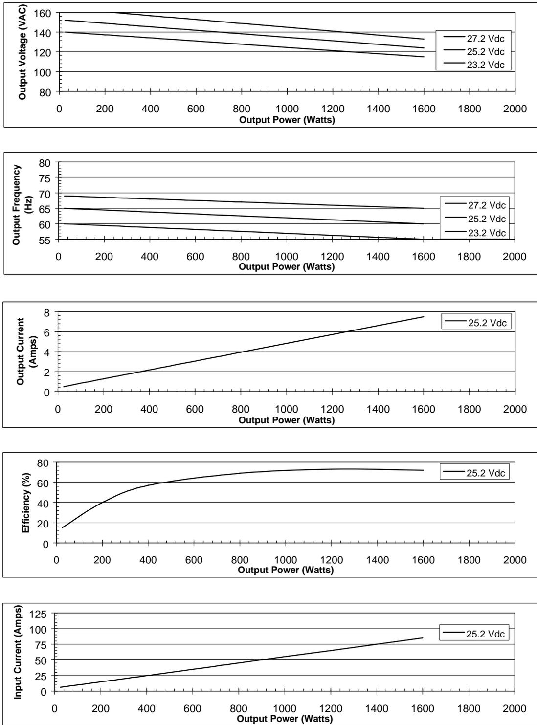
Figure 11-4: Performance Curves for DA24L-1600A Redi-Line Generators
