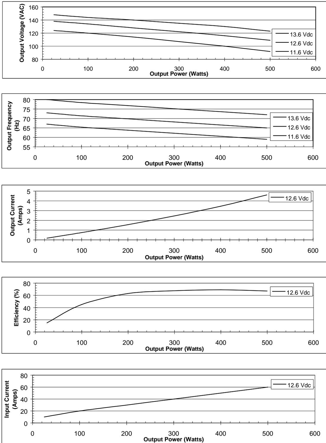
Figure 11-1: Performance Curves for DA12A-500A Redi-Line Generators
