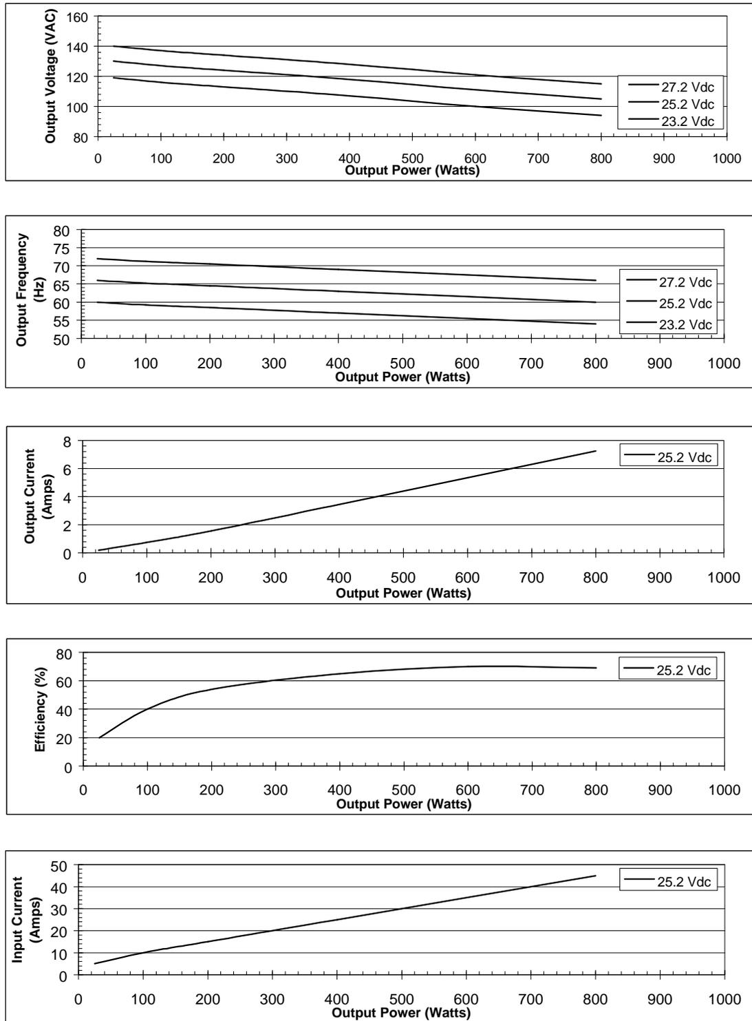
Figure 11-3: Performance Curves for DA24A-800A Redi-Line Generators
