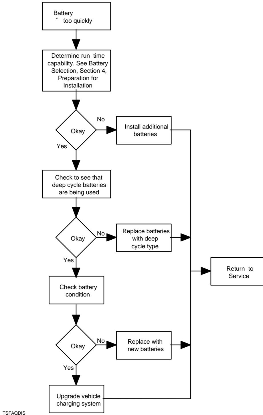
Figure 7-9. Battery Discharges Too Quickly
