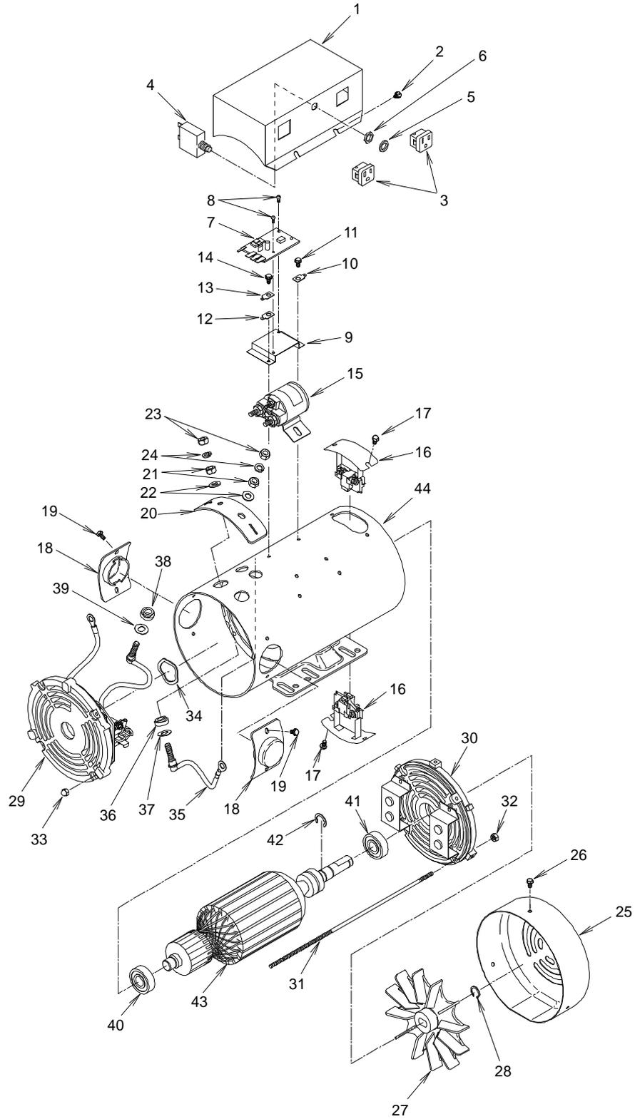
Figure 10-7: 24-Volt Large Frame Generator, Earlier Version
