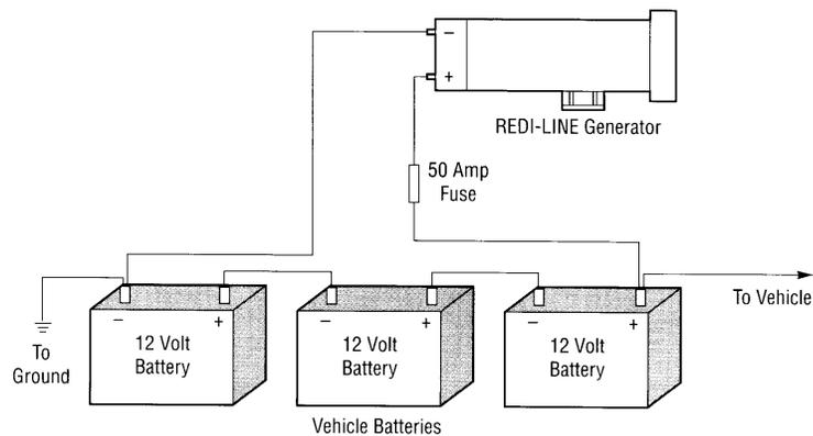
**Figure 4-9: Infrequent Use with Varying Loads**
