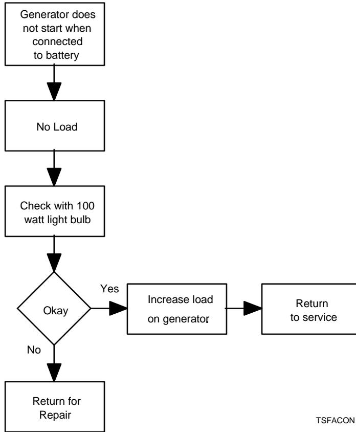
Figure 7-4. Generator Does not Start When Connected to Battery
