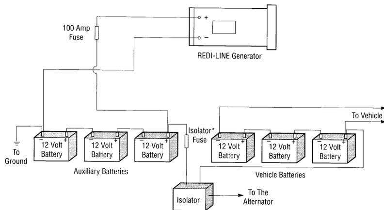
Figure 4-12. Frequent Use with Varying Loads
