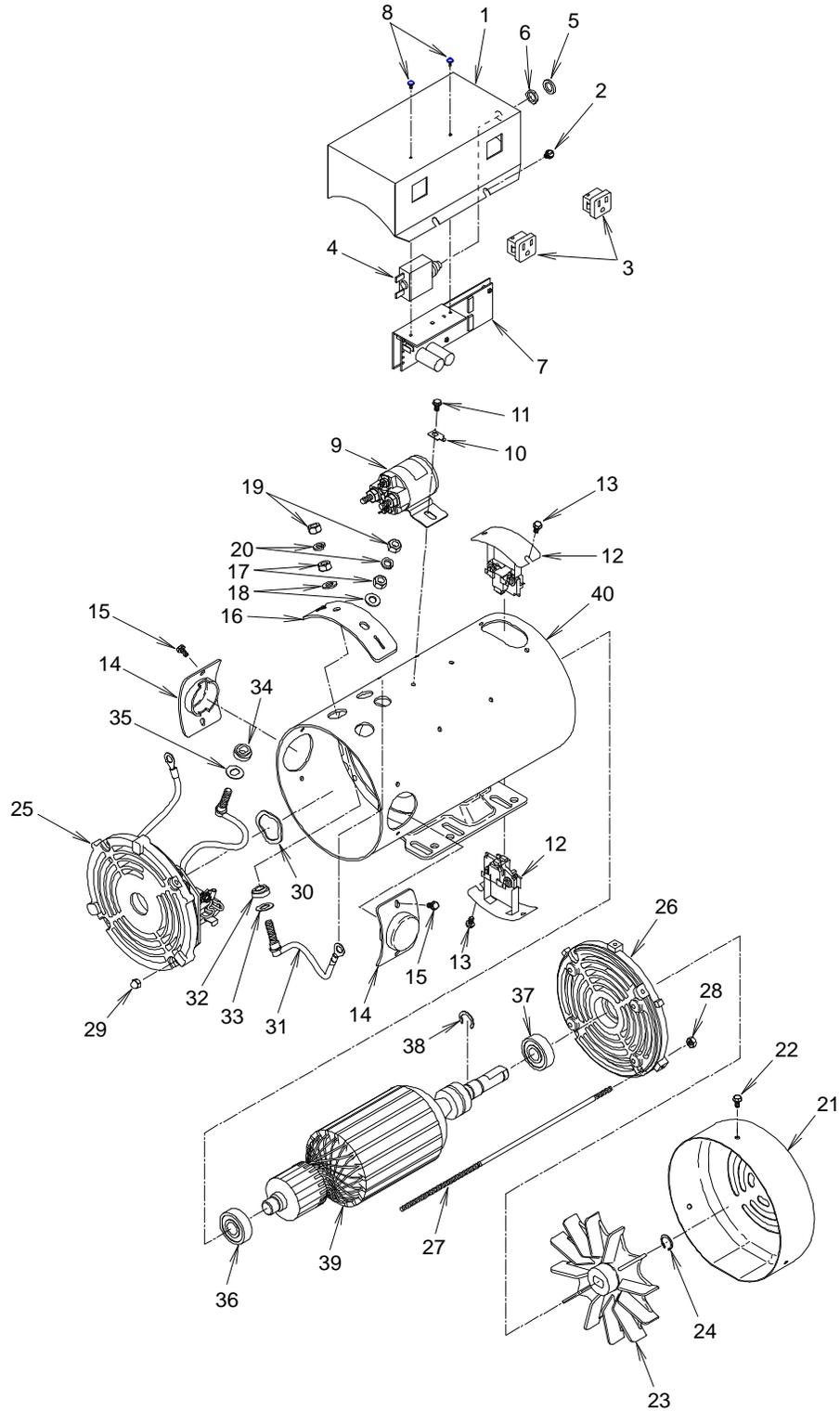
Figure 10-8: 24-Volt Large Frame Generator, Current Version, continued
