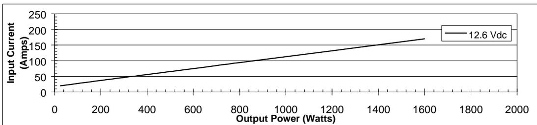
Figure 11-2: Performance Curves for DA12L-1600A Redi-Line Generators
