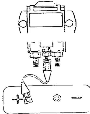
Figure 8-7. Jumper Connection - Large Frame Unit
