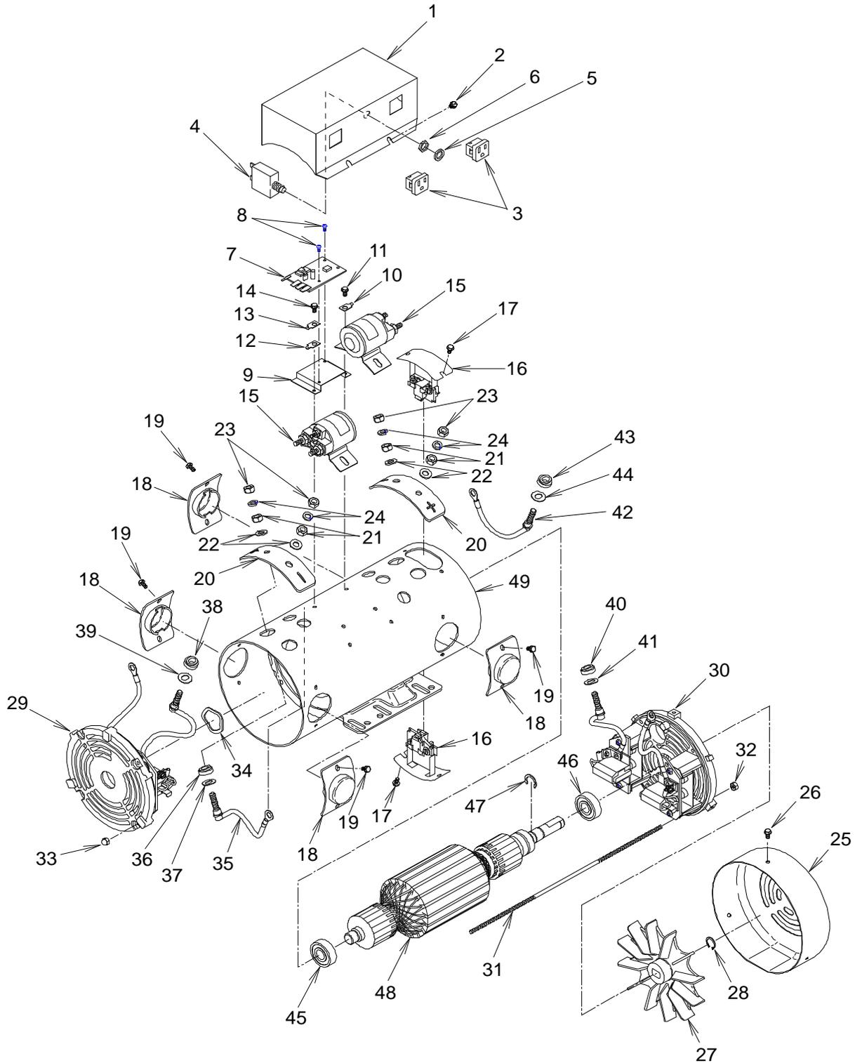
Figure 10-4: 12 Volt Large Frame Generator, Earliest Version
