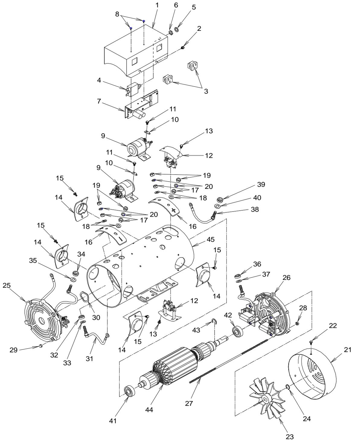
Figure 10-6: 12-Volt Large Frame Generator, Current Version
