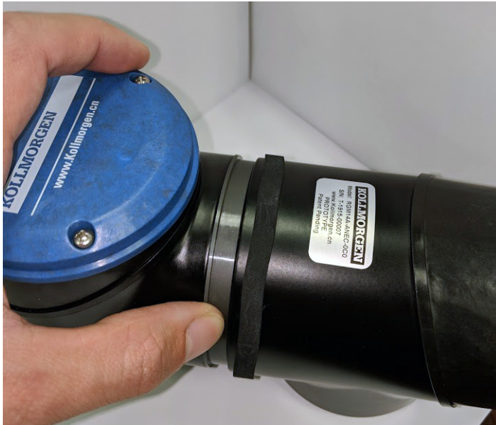
Figure 10: The plastic ring is slid over the fasteners.
