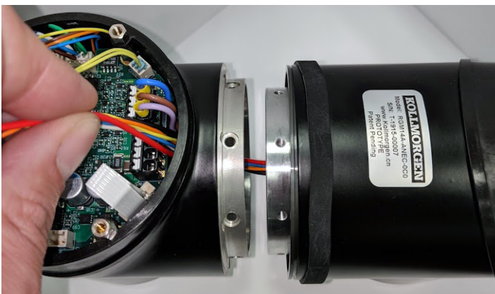
Figure 7: Keep wires taut to avoid pinching
