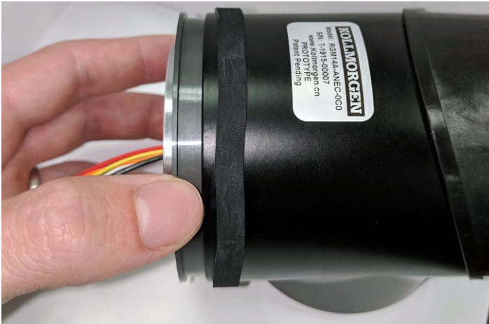
Figure 5: The plastic ring is placed in the RGM device.
