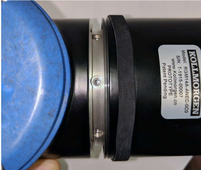
Figure 8: Screw holes are aligned.
