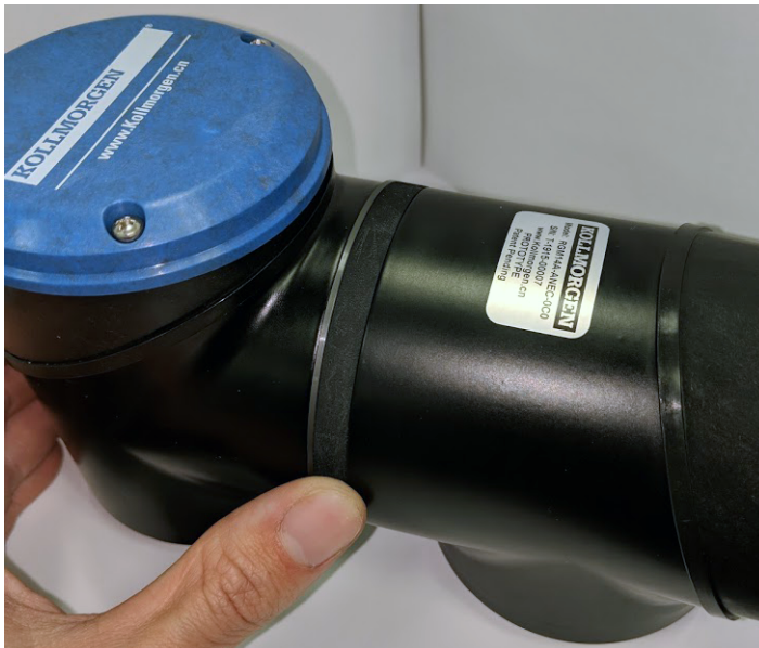
Figure 11: The flexible band secures the plastic ring in place.
