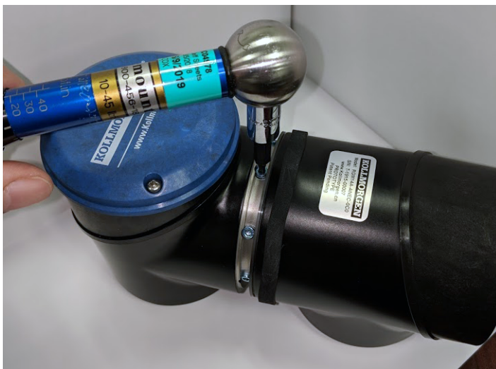
Figure 9: Tighten the screws to the appropriate torque rating.
