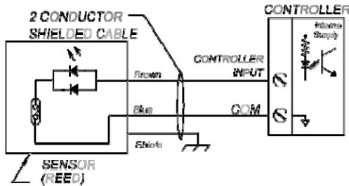
**Note:** The black wire in Quick Disconnect cables is not used with any version of the PSR (Reed) sensor. In the above drawing, only the blue wire, brown wire, and shield are connected.
