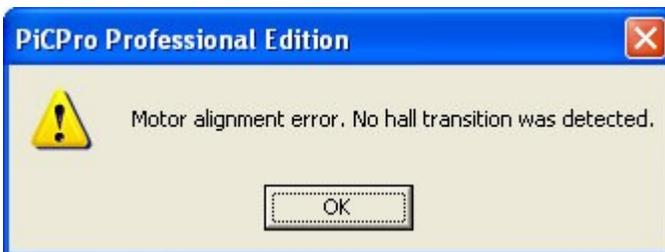
Click **OK** to continue. Make sure the hall sensors are connected correctly to the drive.
