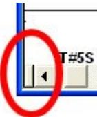
4. When the arrowhead changes to the double line/double arrow, click the button and drag the vertical line into your ladder and release.
