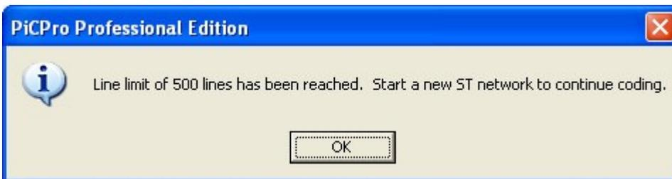
At this time the network will have to be split and a new ST network started. If you want to continue writing the current structured text network, it must be continued in a new network. Any loop or IF/THEN constructs must be closed in the first ST network; they can not be continued in the next network.
