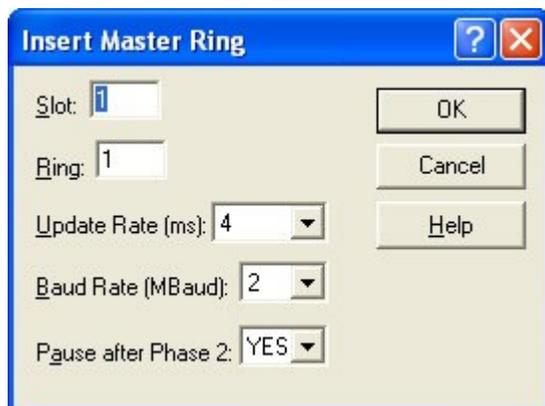
2. Enter the Slot number (3-13) identifying the slot in which your SERCOS module is installed in the control rack.
