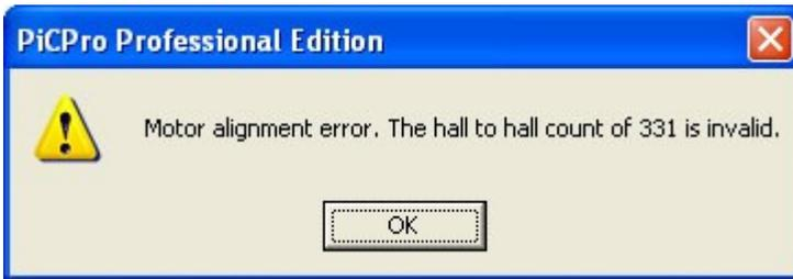
Click **OK** to continue. Make sure the counts per rev and number of poles are correct in the motor data file.
