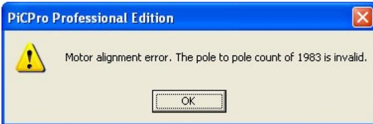
Click **OK** to continue. Make sure the counts per rev and number of poles are correct in the motor data file.
