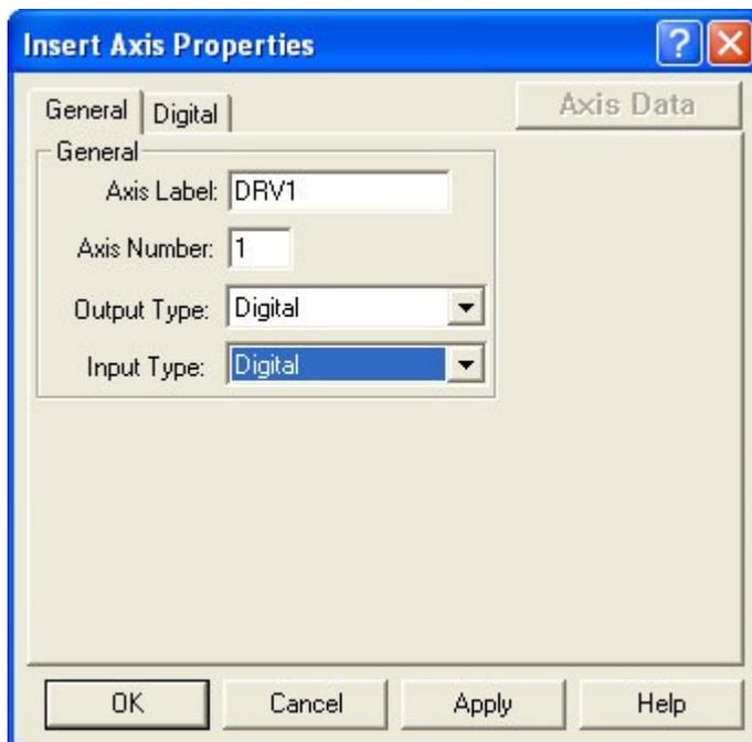
**Virtual** output is also selectable for **Output Type**:. When **Virtual** is selected for **Output Type**:, Input Type: changes to **Virtual**.
