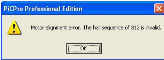
Click **OK** to continue. Make sure the hall sensors are connected correctly to the drive.
