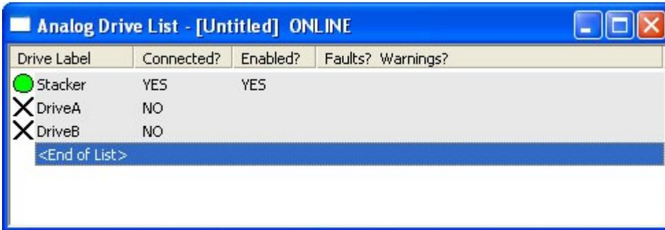
In the ONLINE Drive List view, only one analog interfaced digital drive can be connected at a time.
