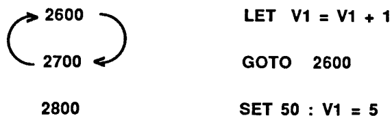
Figure 4-20 Incorrect GOTO Usage
