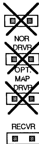
Figure 2-5 Extension Rack Jumper Position
