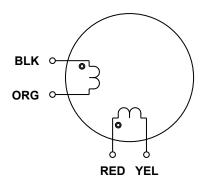
**Note:** Because PMX series does not include any 8-lead configurations, Kollmorgen does not differentiate between bipolar parallel or series within PMX series nomenclature. All 4-lead are simply stated as bipolar. All bipolar winding specifications in this guide represent simple 4-lead connection shown above.
