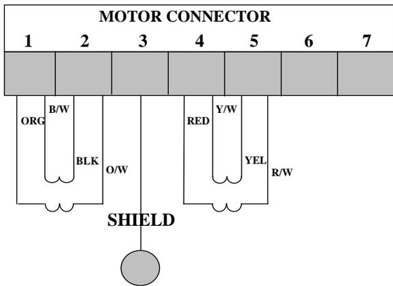
**8 LEAD MOTOR (HALF WINDING)**
