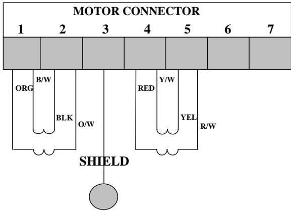
**8 LEAD MOTOR (HALF WINDING)**
