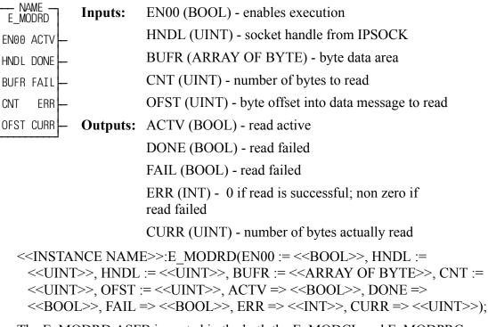
The E\_MODRD ASFB is nested in the both the E\_MODCL and E\_MODPRC ASFBs and is used to read data on the TCP connection.
