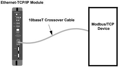
If you are communicating over a plant network you can connect the G&L to an Ethernet HUB using a 10baseT straight cable or a 10Base2 BNC cable. The Modbus/TCP Device is then connected to an Ethernet HUB using a 10baseT straight cable. Both of the Devices would then be connected to the plant network.
