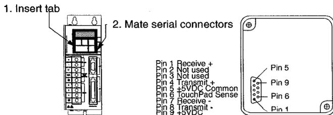
3. Power-up the drive. Installing the TouchPad defaults the drive to the following settings:
