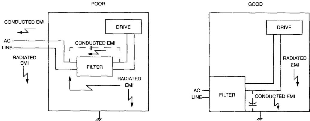
When multiple power cables enter an enclosure, an unfiltered line can contaminate a filtered line external to the enclosure. Therefore, all lines must be filtered to be effective. The situation is similar to a leaky boat. All the holes must be plugged to prevent sinking.
