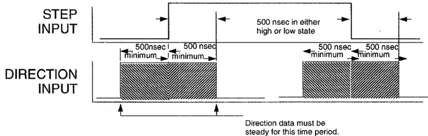
**Figure 6.32 External Step/Direction Interface via TTL Differential Line Drivers**
