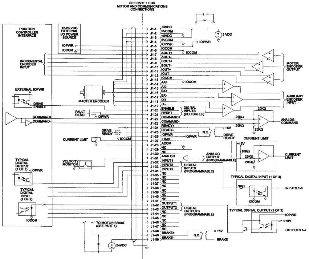
**DSM Interface Connection Diagram - J1**
