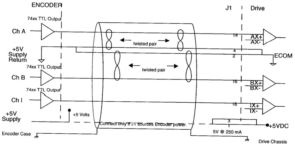
**Figure 6.30 Single-Ended Encoder Interface via Open Collector Transistor with 5 VDC to 12 VDC Pull-up (not recommended)**
