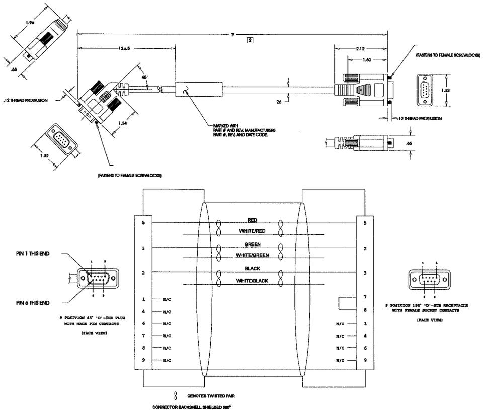
Figure B.4 J5 to J5 Serial Interface Cable (P/N 502-04021)
