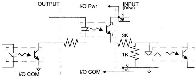
**Figure 6.7 Drive Input Connected to Sourcing Output**
