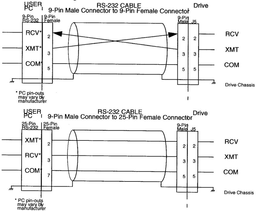
2. Verify the computer can communicate with the drive by performing the following:
