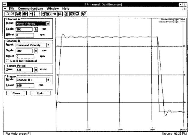
Figure 9.5 Overdamped Signal
