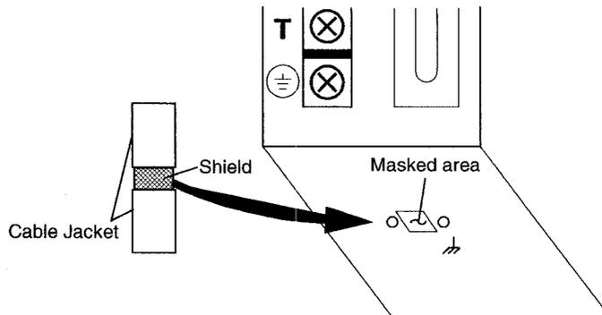
Power cable shield termination clamp on bottom of DSM 007, DSM 015 and DSM 030
