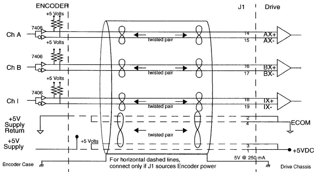
**Figure 6.27 Complementary Encoder Interface via Standard TTL Logic**
