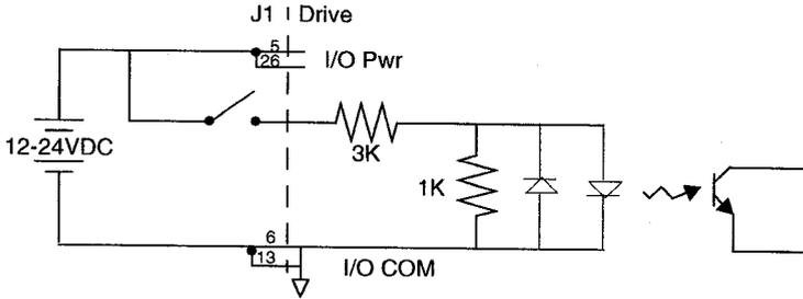
Figure 6.3 Drive Input Connected to an Opto-Isolator
