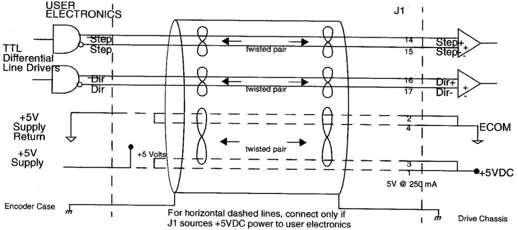
**Figure 6.33 External Step/Direction Interface via Single-Ended TTL Line Drivers (not recommended)**
