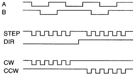
The drive may be electronically geared by a remote signal. Electronic gearing may be driven by any of the following three signals:
