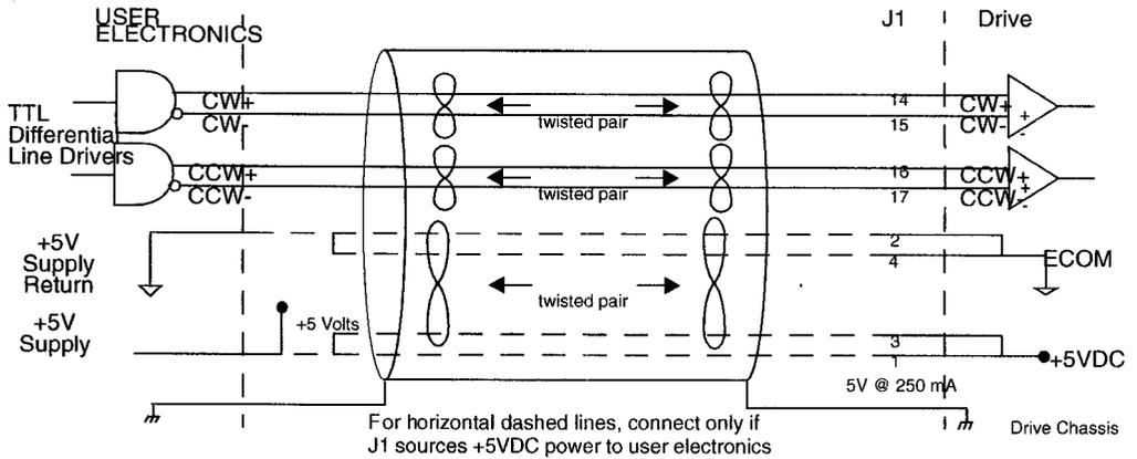
**Figure 6.35 External CW/CCW (Step Up/Step Down) Interface via Single-Ended Line Drivers (not recommended)**
