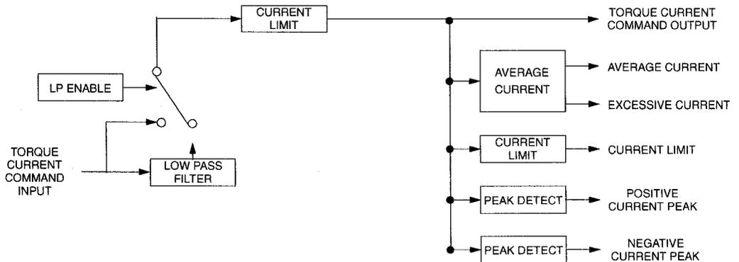
Reducing the value of the P-gain, low-pass filter frequency and the update frequency all have the effect of reducing the servo-motor bandwidth. As long as the resonating frequency is fairly high this will likely be acceptable, but if the resonating frequency is low it may be necessary to modify the mechanics of the system.
