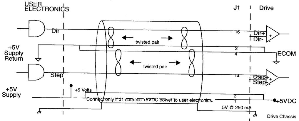
**Figure 6.34 External CW/CCW (Step Up/Step Down) Interface via TTL Differential Line Drivers**
