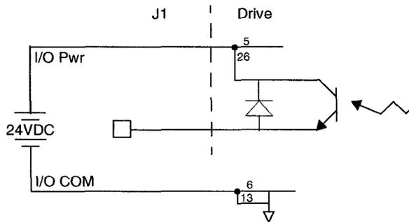
Figure 6.10 depicts a typical applications for the BRAKE/DRIVE ENABLE outputs. Table 6.7 lists the current draw for 24VDC and 90VDC brake coils on Giddings & Lewis motors suitable for use with a DSM 007, 007P, 015, 015P, 030, or 030P.
