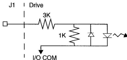
Two discrete input circuit types are available on the J1 connector. Both circuits support logic type interfaces with optically isolated, single ended and active high characteristics.
