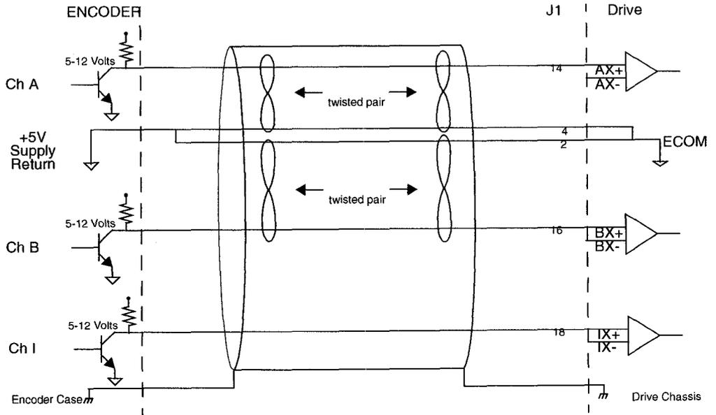
**Figure 6.31 Single-Ended Encoder Interface via Open Collector Transistor with 24 VDC Pull-up (not recommended)**
