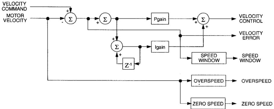
Figure 9.2 Torque Current Conditioning Structure
