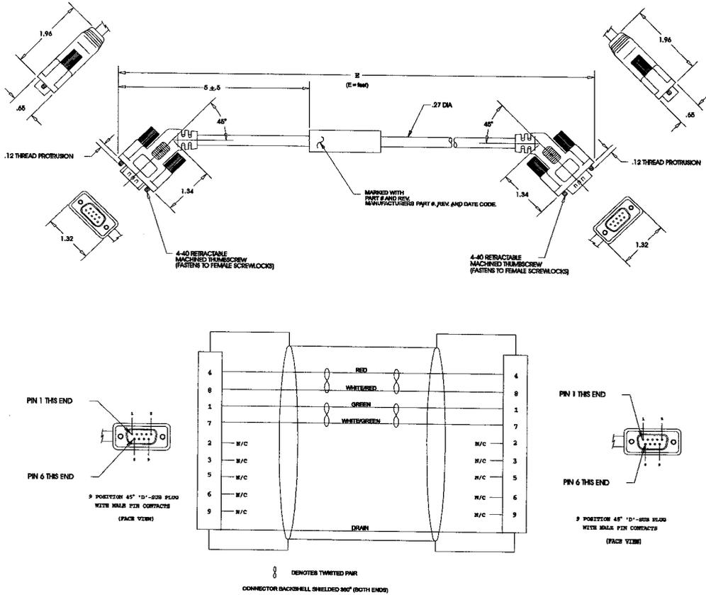
Figure B.5 J5 to No Connector Serial Interface Cable (P/N 401-34423)
