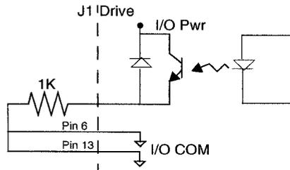
**Figure 6.14 Drive Output Connected to a Switch/Relay**
