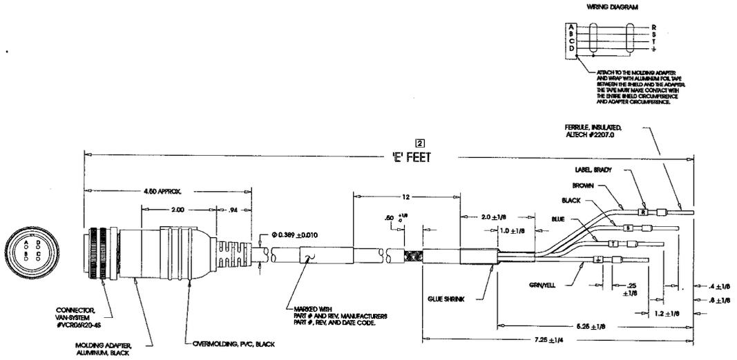
Figure B.13 6000 FSM, HSM or SSM Series Power Cable (P/N 401-34415)
