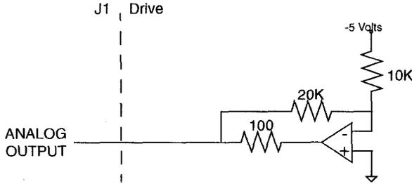
A selectable output is available for monitoring by the user: ANALOG 1 (J1-31).
