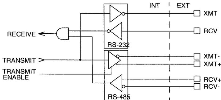
The serial interface of the drive uses the standard NRZ asynchronous serial format, and supports both the RS-232 and the four wire RS-485 communications standards.
