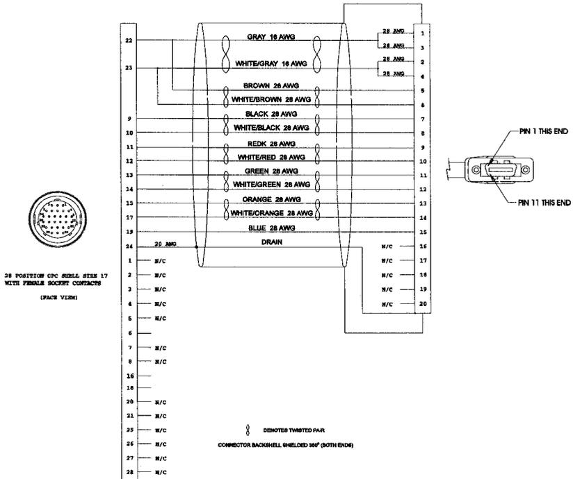
Figure B.9 No Connector to YSM Series Encoder Cable (P/N 401-30253)
