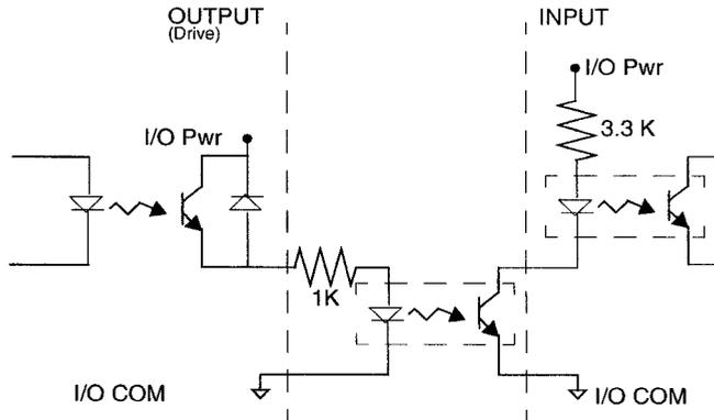
**Figure 6.17 Drive Output Connected to Active High (Sinking) Input**
