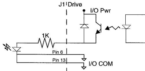
Figure 6.13 Drive Output Connected to a Resistive Load
