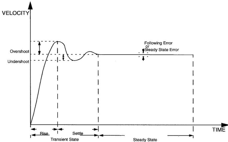
Figure 9.4 Underdamped Signal
