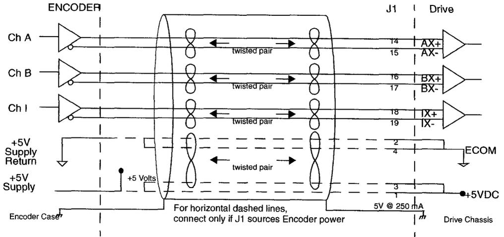
**Figure 6.26 Complementary Encoder Interface via 7406 Line Drivers with Pull-up Resistors**
