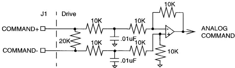
The analog command signal to the drive has a range of  $\pm 10$  Volts. The signal is either a torque or a velocity command, depending on the software configuration of the drive. The differential input is processed by a 14 bit analog to digital converter (ADC) to produce a digital value.
