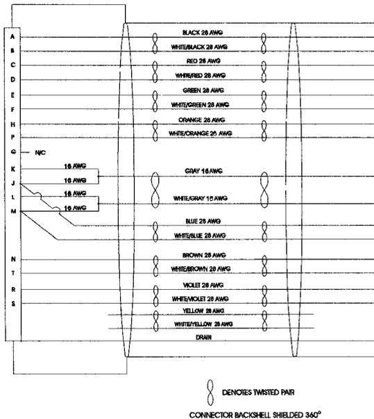
Figure B.7 J2 to FSM, HSM or SSM Series Encoder Cable (P/N 401-4407)
