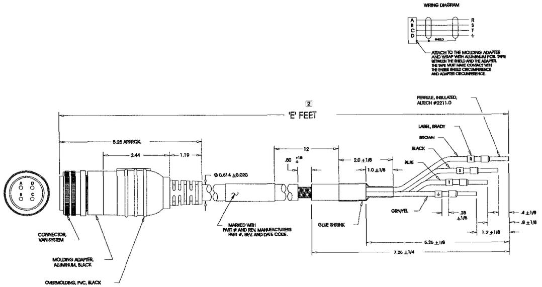
Figure B.14 YSM Series Power Cable (P/N 401-30232)
