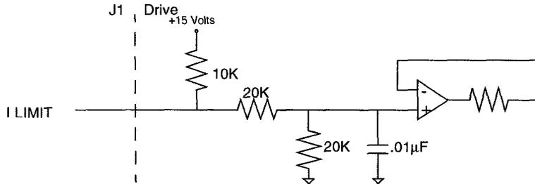
ILIMIT limits the current, which provides torque, to the motor. The range is 0 to +10 Volts (where 10 Volts corresponds to maximum drive current). The analog I LIMIT signal is converted into a digital word by a 10-bit ADC (analog to digital converter). If the I LIMIT input is *not* connected, current is not limited.
