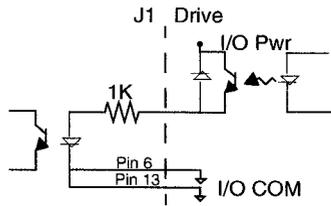
Figure 6.12 Drive Output Connected to an LED Indicator
