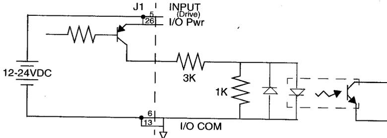
**Figure 6.5 Drive Input Connected to Active Low Output using a Switch/Relay**
