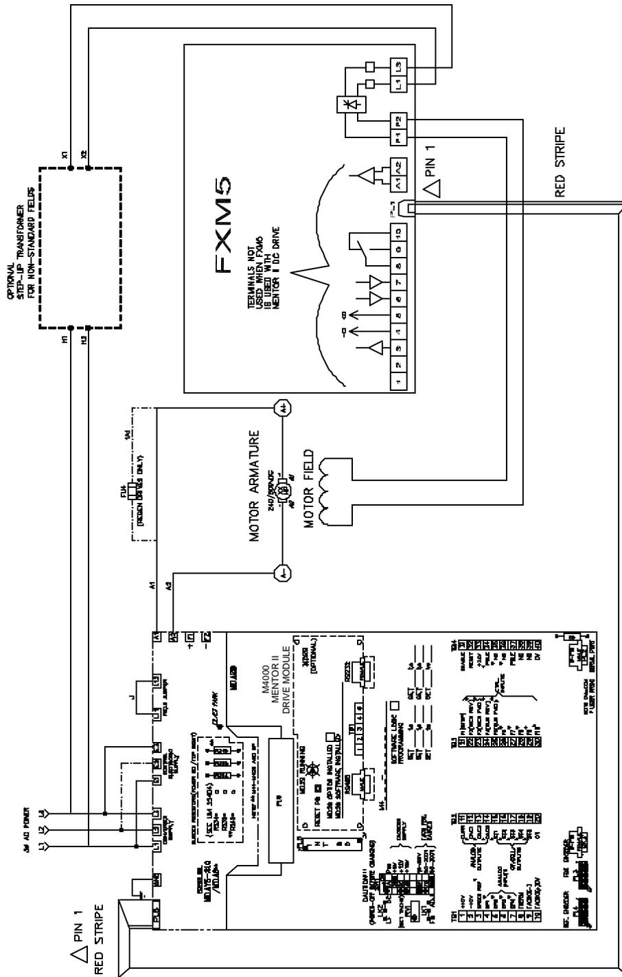
FXM5 CONNECTION DIAGRAM FOR USE WITH M4000 DRIVE
