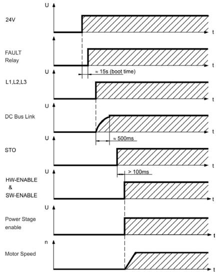
Fault F602 occurs when STO ( $\Rightarrow$  p. 52) does not have current when HW enable becomes active.
