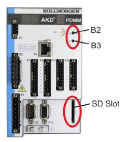
The backup/restore operations (AKD PDMM to SD or SD to AKD PDMM) will not be possible if an application is running.
