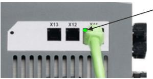
LED is green if drive is connected through a network device.
