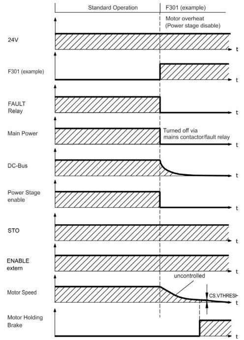
If velocity drops below threshold CS.VTHRESH or timeout occurs the motor holding brake is applied ( $\rightarrow$  p. 103). Set parameter MOTOR.BRAKEIMM to 1 with vertical axes, to apply the motor holding brake immediately after faults.
