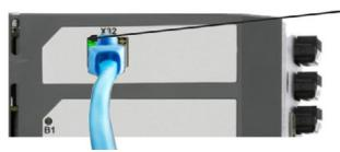
LED is green if drive is connectec through a network device.
