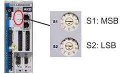
The rotary switches on the front of the AKD (S1&S2) correspond to the CAN node address. The S1&S2 switches also correspond to the IP address setting of the drive. Both CAN and IP network address schemes have to be configured to account for this dependence if both TCP/IP and CAN networks are running at the same time in an application. Example:
