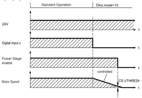
If velocity drops below threshold CS. VTHRESH or timeout occurs brake is applied ( $\rightarrow$  p. 103).
