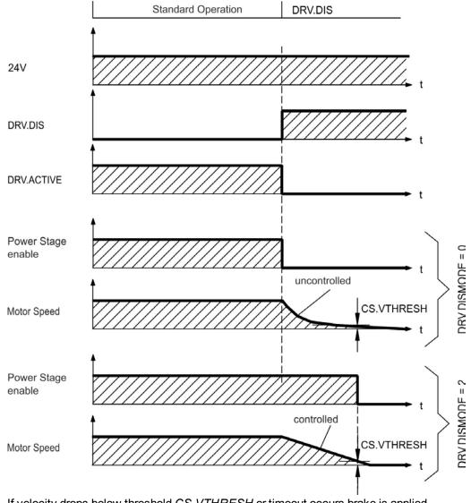
If velocity drops below threshold CS. VTHRESH or timeout occurs brake is applied ( $\rightarrow$  p. 103).
