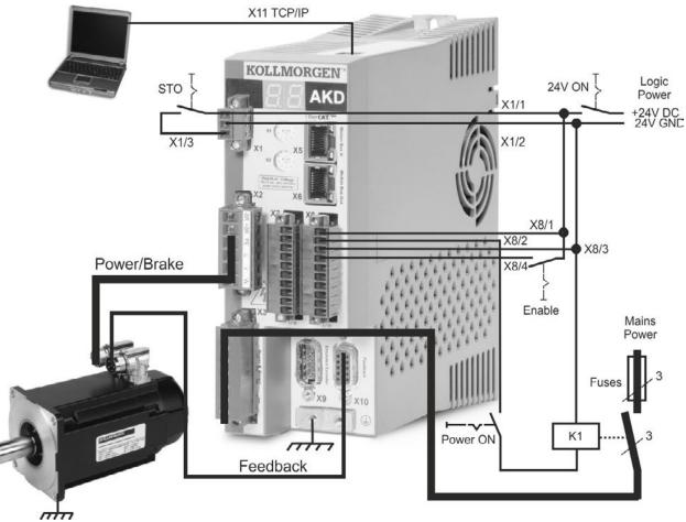
When connecting the AKD directly to a PC, static IP addressing (not 00) is recommended.
