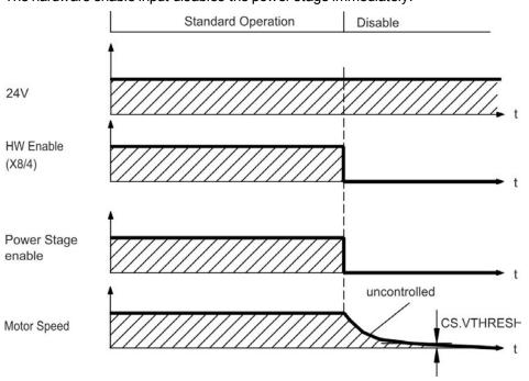
If velocity drops below threshold *CS.VTHRESH* or timeout occurs the motor holding brake is applied ( $\rightarrow$  p. 103). Set parameter MOTOR.BRAKEIMM to 1 with vertical axes, to apply the motor holding brake immediately after Hardware Disable.
