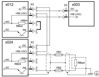
Without DC Bus fuses, other devices can become damaged or destroyed if, for example, a device fails due to an internal short circuit. If multiple drives are connected in parallel, then it is usual to insert DC Bus fuses ( $\rightarrow$  p. 37.) between groups of drives (with a group consisting of two or three devices, depending on the current) in order to limit any possible resulting damage. Fuses cannot avoid damage by current peaks completely.
