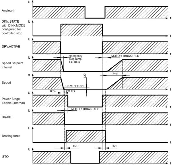
The speed setpoint of the drive is internally driven down an adjustable ramp (CS.DEC) to 0 V. With default values the output for the brake is switched on when the speed has reached 120 rpm (CS.VTHRESH) for at least 6 ms (CS.TO). The rise ( $t_{brH}$ ) and fall ( $t_{brL}$ ) times of the holding brake that is built into the motor are different for the various types of motor.
