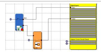
**Note**: When editing the associated inPort element, the connection with the start element is deleted and cannot be restored automatically. It must be subsequently supplemented manually.
