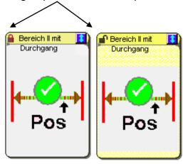
When inserting a new group frame the switch "Disable group management" is set to unlocked state by default. After closing the group editor the drawn frame appears in the logic diagram and represents the active area of the group.
