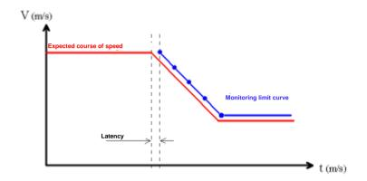
When activating the SLS, the parameterized SSX is automatically activated via the SLS. The SSX monitors the ramp course of the speed. If the actual speed is lower than the SLS threshold, the SLS will take over the further monitoring, until the SLS is deactivated again.
