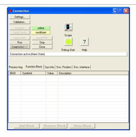
(**Scope**): Opens the <u>Scope monitor</u> dialog. This enables the representation of various process data.
