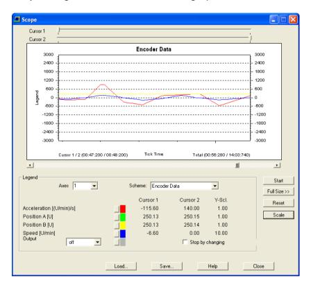
**Note**: With an active Scope Monitor the output of debugging of process image and logic diagram is hidden and the diagnostics tabulator is blocked throughout the connection dialog. These data cannot be made available in this mode.
