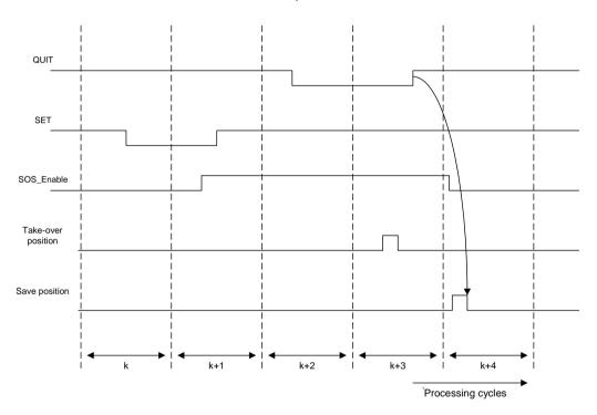
The sequence is time monitored and triggers an ALARM if the expectations are exceeded.
