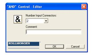
**Note**: The number of inPort connectors can only be reduced in case of free connectors. If all connectors have linkages assigned, these must be deleted beforehand.
