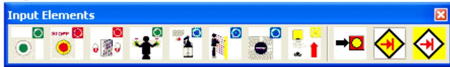
The inPort elements create the digital connection between one or several connected sensors and/or further lower-level switching devices in the **KSM System**. Each inPort element, except the mode selector switch, provides one logic output signal "0" or "1" for further processing in the PLC.
