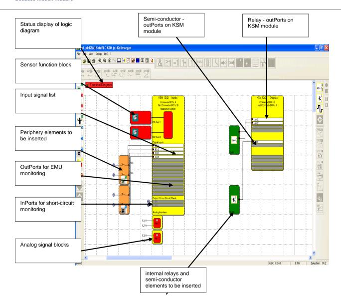
If function blocks are inserted into the terminal diagram, the elements will automatically be wired. In some instances it may happen, that the connections are unfavourably displayed. However, this does not affect the function! When moving the corresponding block, the connecting wiring will be redrawn and may appear more distinctly.
