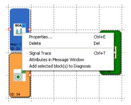
**Tip**: The attributes of all functional modules can be copied using the command "Attributes into Message Window". In this case no functional module must be selected.
