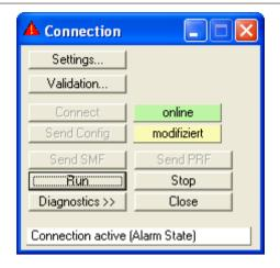
**Send configuration:** Transmits the configuration of the logic diagram to the KSM-system. This is only possible in "Stop" mode.
