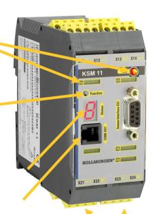
Terminal blocks for input / output signals
