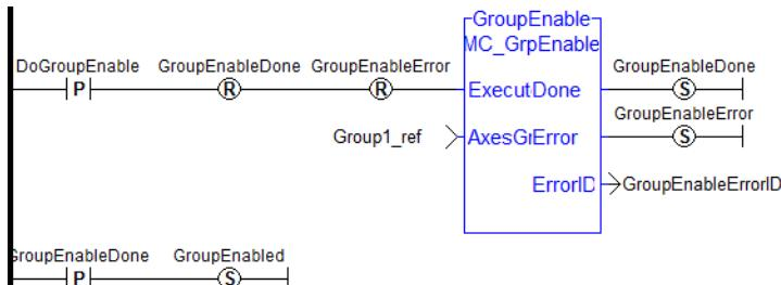
To remedy this, the following code uses the SET and RESET of a Boolean (i.e. EnableRequest) to provide a way to detect each successful execution of the function block:
