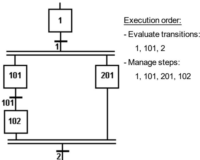
In case of a divergence, all conditions are considered as exclusive, according to a "left to right" priority order. It means that a transition is considered as FALSE if at least one of the transitions connected to the same divergence on its left side is TRUE.
