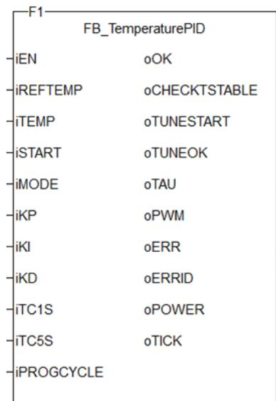
Figure 5-28: The TemperaturePID user-defined function block
