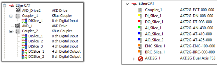
Figure 4-106: EtherCAT Network - Logical View. K-Bus on left, E-Bus on right
