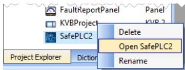
2. SafePLC2 will be launched and the Safety Project will be opened. SafePLC2 automatically populates the safety devices from the EtherCAT Safe topology defined in the KAS IDE.
