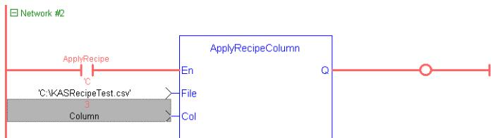
Column 3 corresponds to column E in the Excel sheet because this parameter is 0 based
