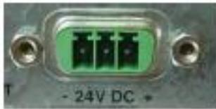
**Figure 3.1** DC-connector (without Phoenix plug terminal)
