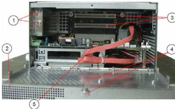
1. Screws to secure the expansion
