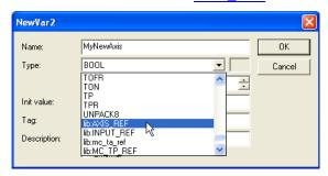
Figure 5-18: PLCopen Axis - New Instance of AXIS REF
