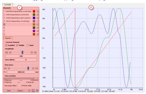
Figure 7-23: Example of using the Oscilloscope
