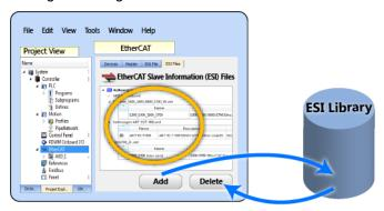
**Figure 5-115: Adding/Deleting** — Adding or deleting an ESI file from the KAS IDE affects KAS's internal library of ESI files.
