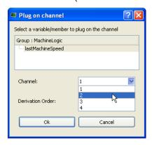
Figure 5-68: Plugging a PLC Variable - Parameters
