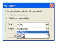
Figure 5-97: Define Type and Scope of the Variable
