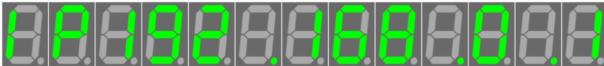
Figure 7-1: Example of the IP sequence by the 7-segment display.
