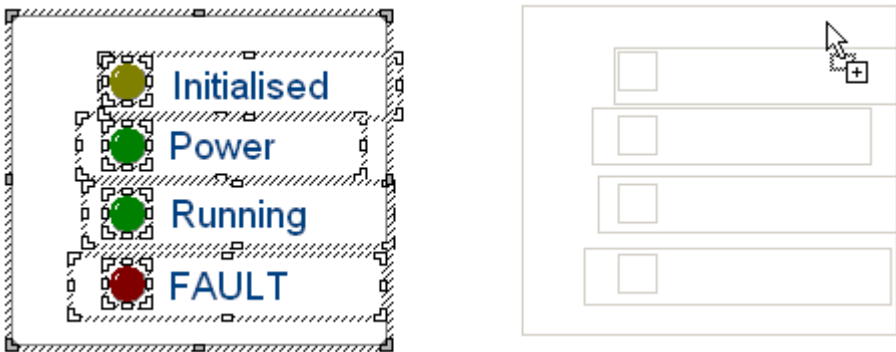
Figure 8-34: Control Panel - Selection of Controls
