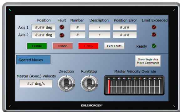
Figure 2-9: Hardware to Display the Human-Machine Interface
