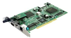
Figure 2-14: PCI Interface Card
