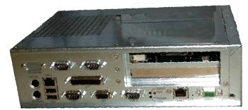
Figure 2-10: Programmable Automation Controller
