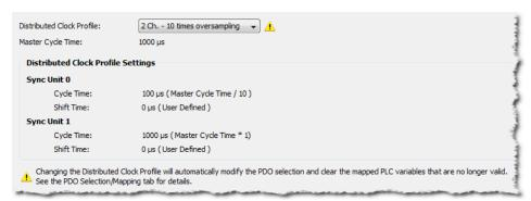
Figure 4-117: Example of a device with oversampling.
