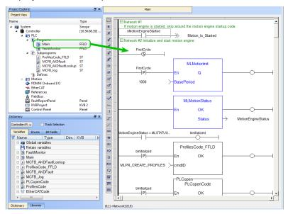
Figure 7-55: PLCopen Template with FFLD - Main
