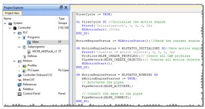
Figure 7-45: PLCopen Template with ST - Main
