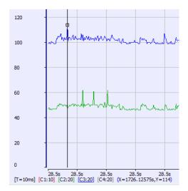
This shows the MotionExec at 62 microsec and the PLCProgExec at 114; there is not much time left over.
