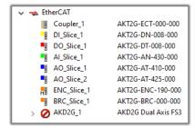
**Figure 4-106:** EtherCAT Network - Logical View. K-Bus on left, E-Bus on right
