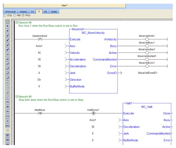
Figure 7-47: PLCopen Template - Step 5 of the Main
