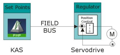
Figure 5-2: Regulation with Remote Drive
