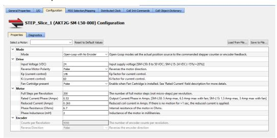
Select a Motor: The drop-down list contains nearly 500 Kollmorgen stepper motor models and their
