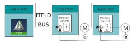
Figure 5-3: Multi-Axis Driven by a Virtual Master
