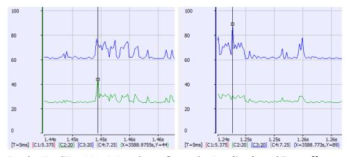
For the "RealTimeMargin" peaks configure the **Amplitude** and **Zero offset** so you can see the trace near zero. In this example the minimum peak (closest to zero) is 69 microseconds. This provides a 28% (69 / 250) Real Time margin which is good.
