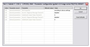
Figure 7-27: Example of configuring sub-modules.
