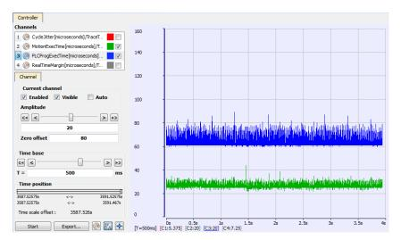
The average time for the MotionExecTime + PLCProgExecTime is 95 (27 + 68 = 95), which is about 38% of the cycle (95 / 250). This is a good value.
