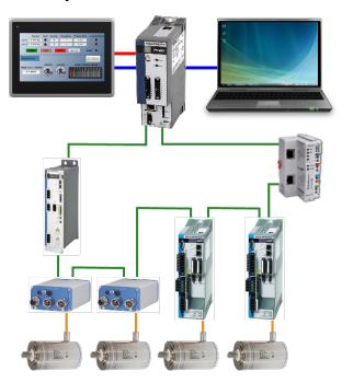
Figure 2-6: Example of Automation System
