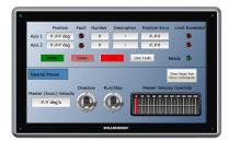
Figure 2-8: Hardware to Display the Human-Machine Interface
