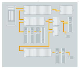
Figure 5-19: Flexible Topology: Line, Tree or Star
