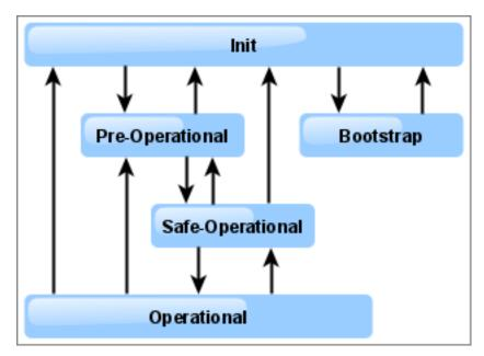
Figure 5-29: EtherCAT State Machine
