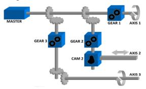
Figure 5-6: Mechanical System
