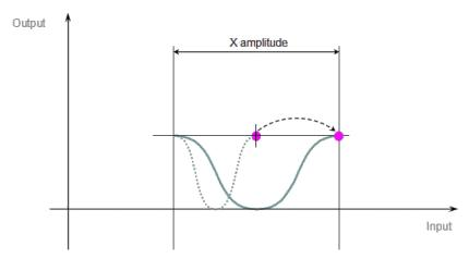
Figure 4-44: Cam Profile Transformation - Step 2
