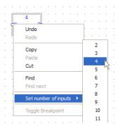
Figure 4-33: Set the Pins Number of the Block
