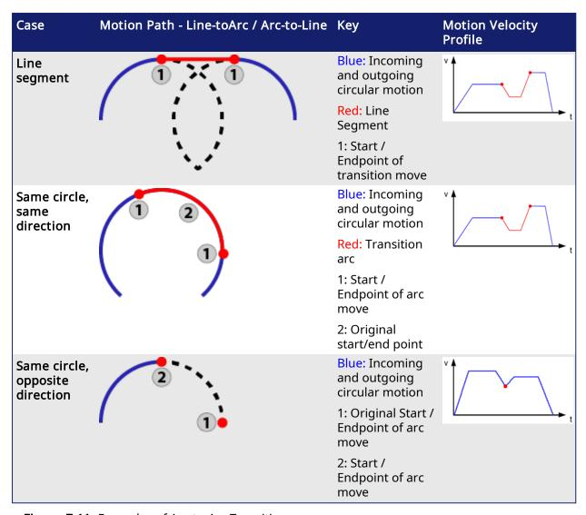
Figure 7-11: Examples of Arc-to-Arc Transitions
