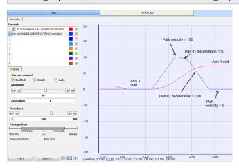
**Figure 7-12:** Oscilloscope Representation of linear coordinated move with a MC\_GrpHalt command called twice
