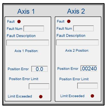
Figure 7-54: PLCopen Template - Fault Report Panel
