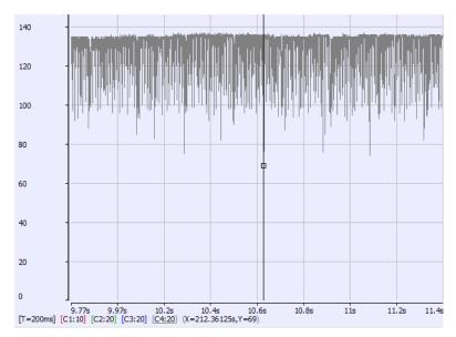
For the "CycleJitter" trace configure the **Amplitude** and **Zero offset** so you can see the trace *centered* at zero. This trace is not too interesting unless a system is misbehaving. A jitter of +/-15 microseconds is acceptable.
