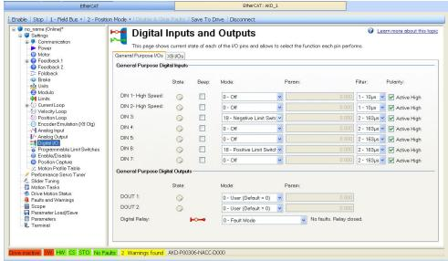
On this screen, you can set the mode of each Digital IO on the drive using the dropdown list in the Mode column. For more information about this view see .
