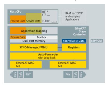
Figure 5-27: Slave Hardware: FPGA with Host CPU
