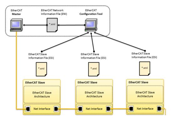
Figure 5-26: EtherCAT Network Architecture1
