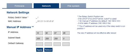
Figure 6-5: Example of a AKD PDMM or PCMM with a manually defined IP address
