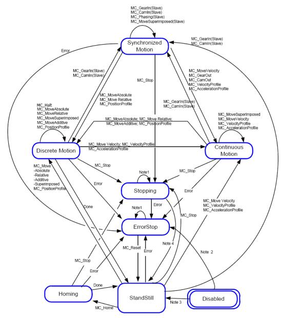
Figure 5-16: Motion State Machine (PLCopen)
