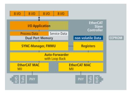
Figure 5-28: Slave Hardware: FPGA with direct I/O
