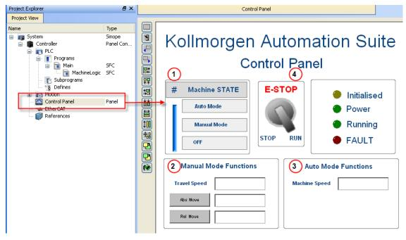
Figure 7-43: PN Template - Control Panel
