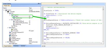
Figure 7-51: PLCopen Template with ST - Main
