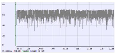
Notice the minimum time is 20 microseconds or 8% Real-Time margin (20 / 250). This is not a comfortable margin for deterministic Real-Time performance.
