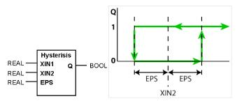
The function block is based on the programming language function block Diagram and has the name Hysterisis. It has three inputs (XIN1, XIN2 and EPS) of datatype REAL on the left, and one output (called Q) of type BOOL on the right-hand side.
