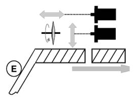
Figure 2-2: Spring Winding
