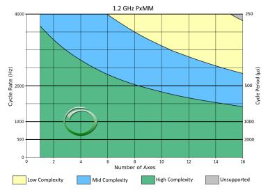
A 12-axis middle-complexity application running at 4 kHz (250us) requires the dual-core 1.2 GHz PxMM.
