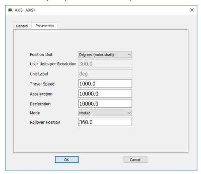
Figure 4-14: Setting Axis Units
