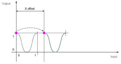
Figure 4-43: Cam Profile Transformation - Step 1
