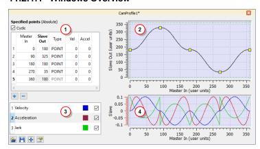
Figure 6-11: Cam Profile Editor Main Window
