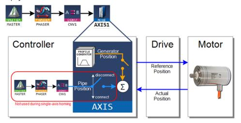
Figure 5-9: Axis Pipe Block Positions
