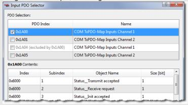
• Device vendors determine the PDO(s), content and possible selection exclusivity. This information is defined inside the device vendor's ESI file. Please contact the device vendor for details about a specific device.
