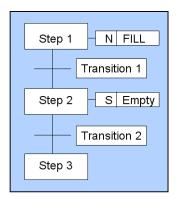
SFC organizes the internal structure of a program, and helps to deconstruct a control problem into manageable parts, while maintaining the overview.
