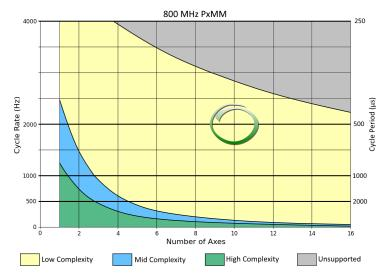
A 4-axis high-complexity application running at 1 kHz (1000us) can be handled by a single-core
