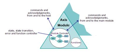
Figure 7-30: Axis Module Description
