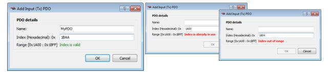
Figure 4-116: Examples of live checking for valid entries.
