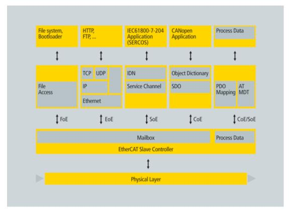
Figure 5-23: Several Device Profiles and Protocols can coexist
