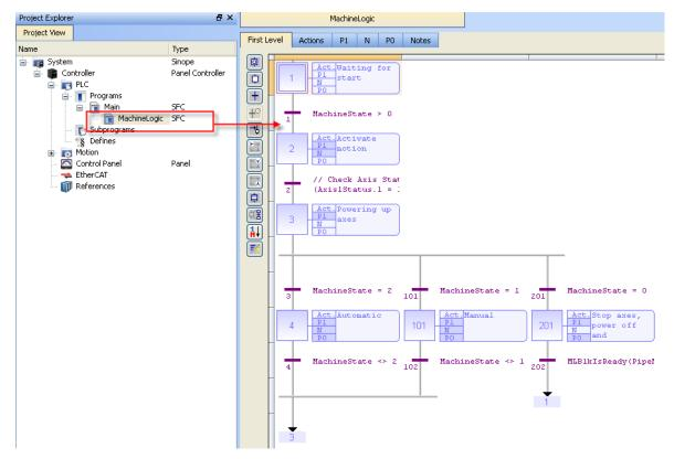
Figure 7-35: PN Template - MachineLogic
