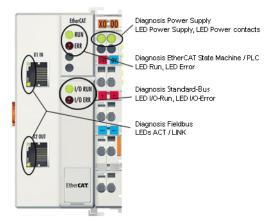
Figure 9-4: ETHERCAT Coupler Diagnostic LEDs
