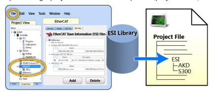
**Figure 4-113: Saving** — When a KAS project is saved, a copy of the ESI file(s) is included in the project file.
