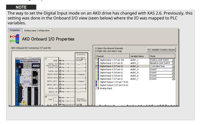
The 'Digital Inputs and Outputs' are now accessed using the new AKD GUI integration inside KAS. This will allow you to save this setting inside the drive instead of pushing it every time the application is started.
