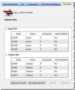
The Input (Tx) and Output (Rx) PDOs are grouped separately. Each PDO table contains the following information:
