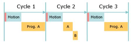
Figure 5-33: Application Overrunning the Basic Cycle
