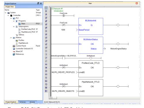
Figure 7-32: PN Template with FFLD - Main
