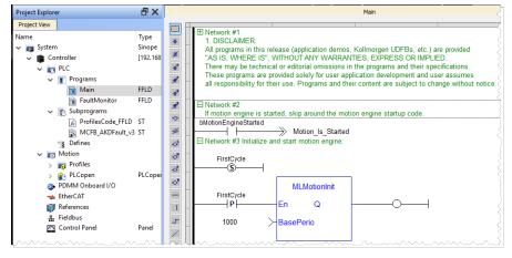
Figure 7-44: PLCopen Template with FFLD - Main
