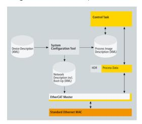
Figure 5-25: Structure of EtherCAT Master Implementation
