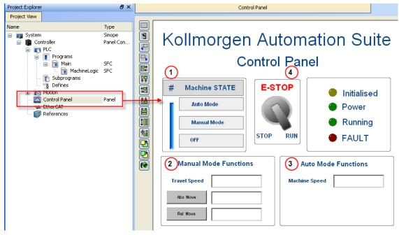
Figure 7-40: PN Template - Control Panel
