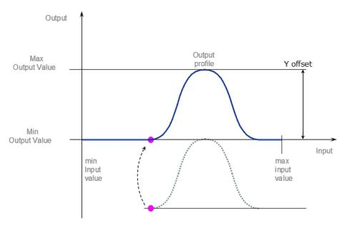
Figure 4-46: Cam Profile Transformation - Step 4
