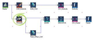
Figure 7-22: Example of using a Pipe Network Trigger block for position capture.
