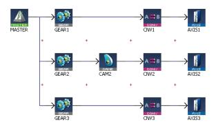
Figure 5-7: Pipe Network Structure
