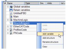
Figure 4-91: Add Variable to a Complex Structure
