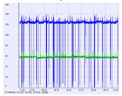
The average MotionExec and PLCProgExec times are 57 + 125 = 182 or 73% (182 / 250) of the Cycle Time. Notice the big spikes on the PLCProgExec?
