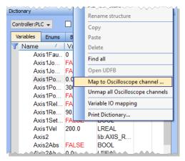
Figure 6-34: Plugging a Probe from the Dictionary
