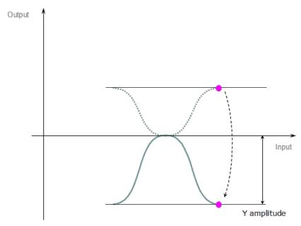
**Figure 4-45:** Cam Profile Transformation - Step 3
