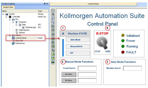
Figure 7-37: PN Template - Control Panel
