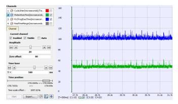
The average MotionExec + PLCProgExec = 50 + 105 = 155 microseconds. This is about 62% (155 / 250) of the cycle time.
