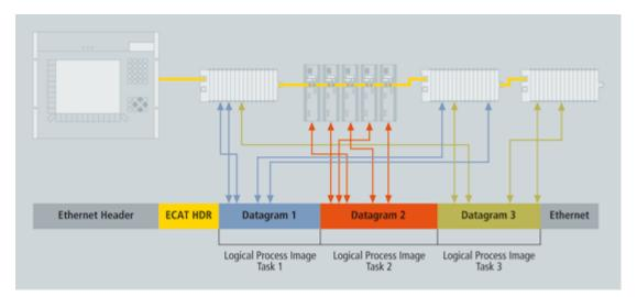
Figure 5-18: Process Data is Inserted in Telegrams
