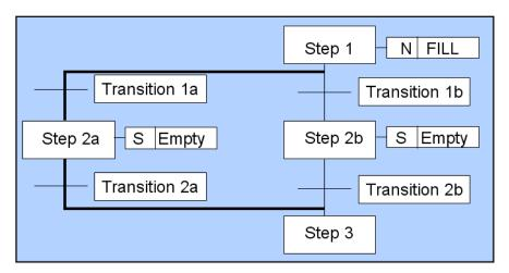
Figure 5-1: Example of a Parallel Sequence in SFC
