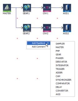
Figure 4-6: PipeNetwork - Add Pipeblock
