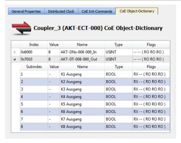
CoE objects can be composed of a simple data type or a complex type. In case of a complex data type, each simple data type composing it has a SubIndex . As shown in the example below, the CoE object can be expanded to show all the subindex's details that are the same as the details for a simple type CoE object.
