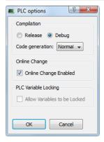
Figure 4-58: PLC Options - Debug Compiling Mode
