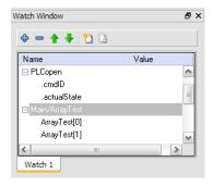
Figure 3-16: Watch Window - Accessing Arrays
