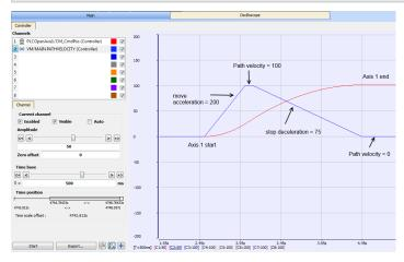
**Figure 7-13:** Oscilloscope Representation of linear coordinated move with a MC\_GrpStop **Exceptions:**
