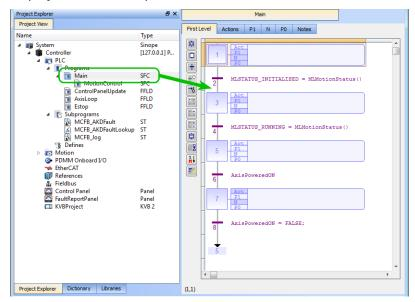
Figure 7-46: PLCopen - Template Main
