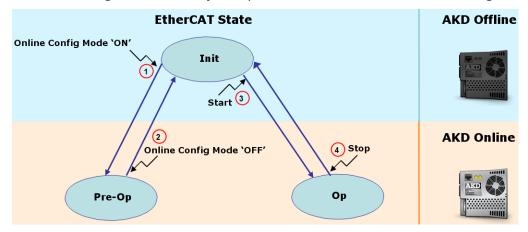
Figure 5-31: AKD Configuration According to EtherCAT State
