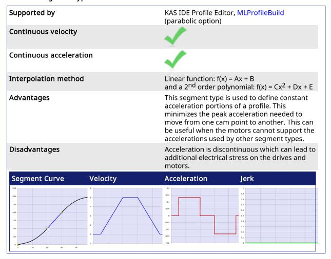
In the example shown, the blue line represents the linear (constant velocity) part of the segment, while the black lines represent the parabolic (constant acceleration) parts of the segment.
