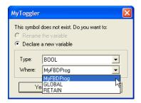
Figure 4-94: Define Type and Scope of the Variable
