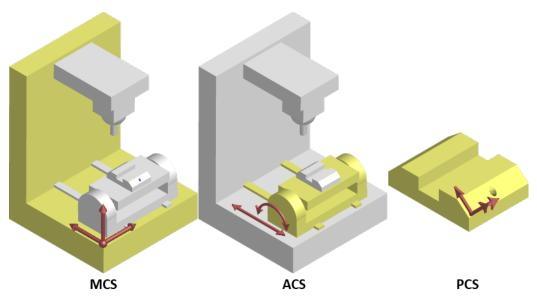
Figure 7-1: Examples of CS types on a machine and part.
