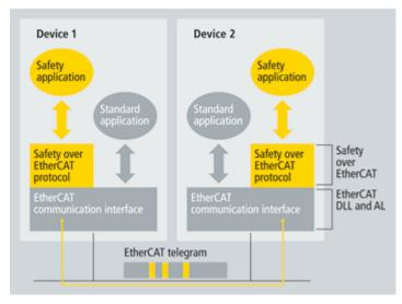
Figure 5-21: Safety over EtherCAT Software Architecture
