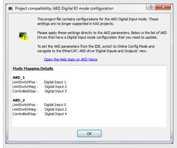
For each drive you will find the list of digital inputs with their specific mode settings. You can copy/paste the content of this text area to a text editor to keep track of them before closing the dialog box.
