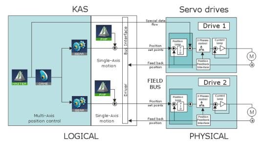
Figure 5-4: Hardware Organization of Motion Functions
