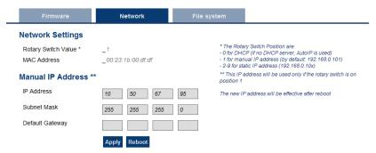
Figure 3-5: Example of a PDMM or PCMM with a manually defined IP address
