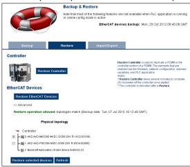
The web server displays the backup and physical topology and indicates the non-compatible drives if the backup and replacement drive are not compatible,.
